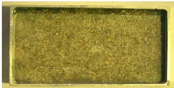
**Fig. 1:** Brass reinforced epoxy composite.
