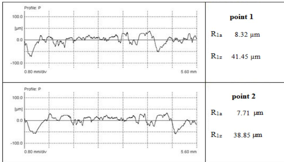
**Fig. 2:** Roughness graph for level 2 (A1, B2, C2).
