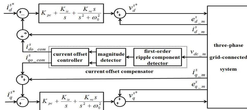
**Fig. 7:** Block diagram of a current control system using the proposed current offset compensator in three-phase grid-connected inverters.
