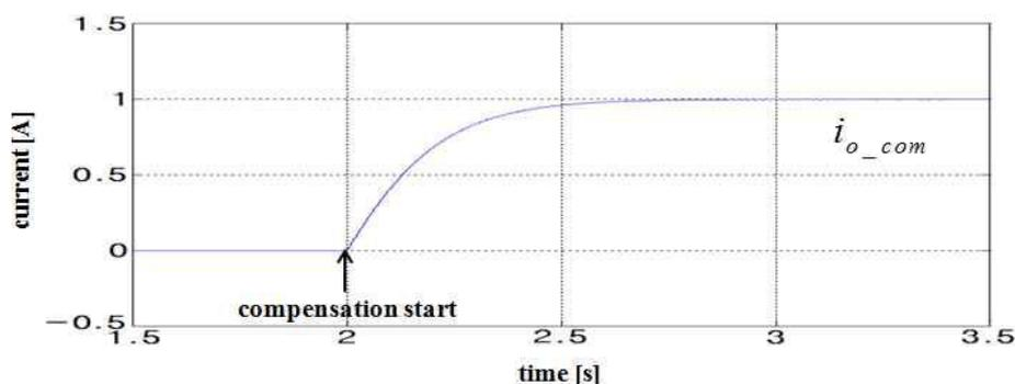
**Fig. 9:** Output of the current offset compensator in single-phase. grid-connected inverters.
