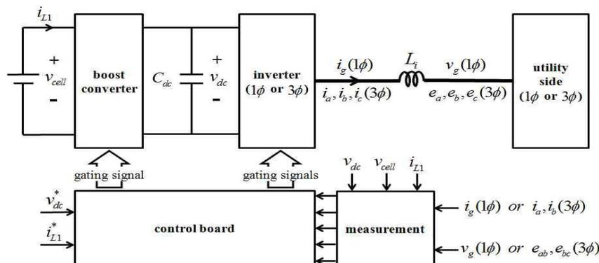
**Fig. 8:** Sample distributed generation system for simulations and experiments.
