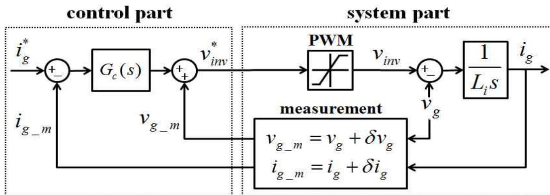
Fig. 1: Block diagram of the current control in measurement in single-phase grid-connected inverters.
