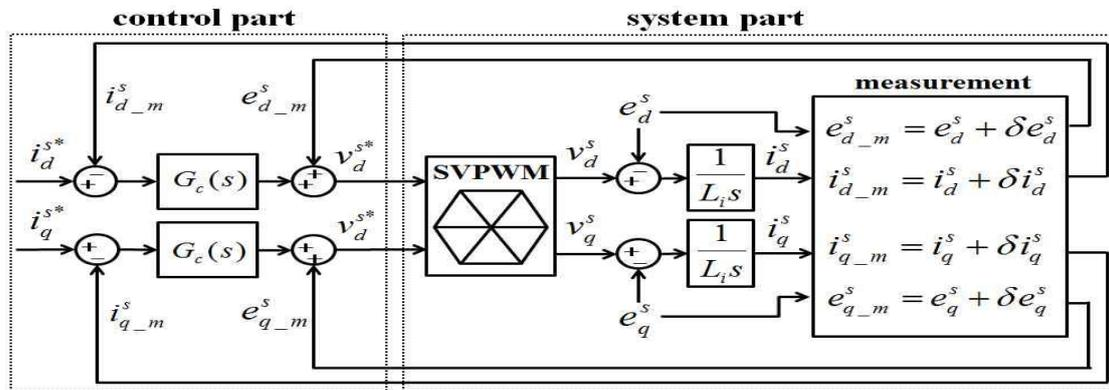
**Fig. 3:** Block diagram of the current control in measurement of three-phase grid-connected inverters.
