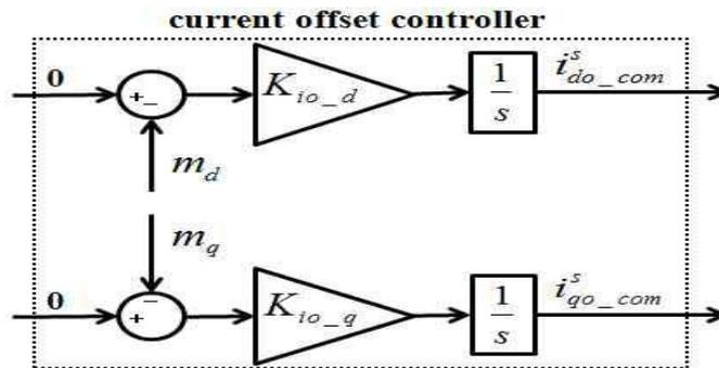
**Fig. 6:** Block diagram of a current offset controller in three-phase grid-connected inverters.
