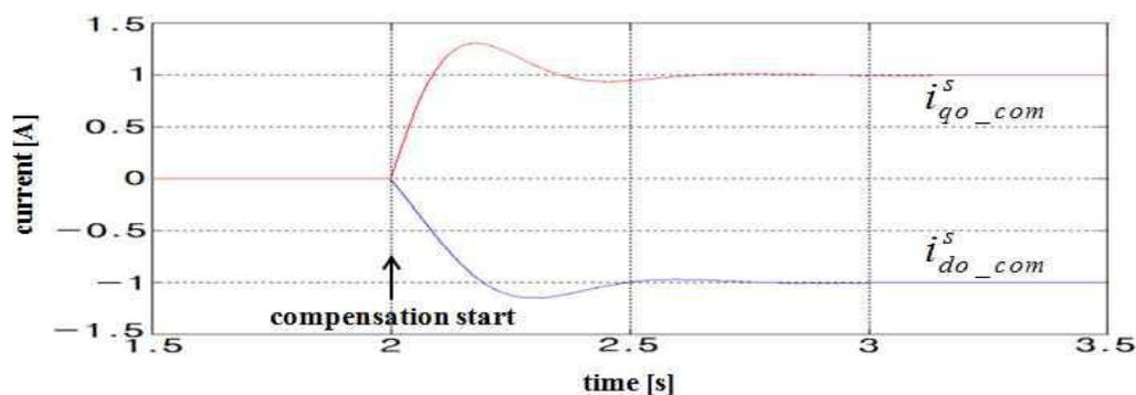
**Fig. 10:** Output of the current offset compensator in three-phase grid-connected inverters
