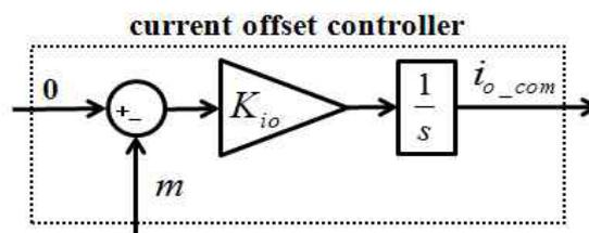
Fig. 4: Block diagram of a current offset controller in single-phase grid-connected inverters.
