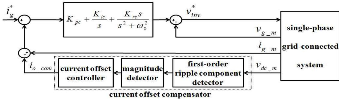
**Fig. 5:** Block diagram of a current control system using the proposed current offset compensator in single-phase grid-connected inverters.
