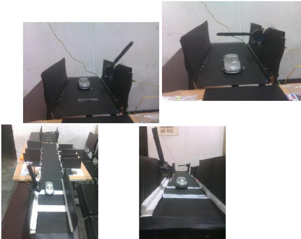
The signal from the sensor circuit enables the motor to rotate clockwise or anti-clockwise.
