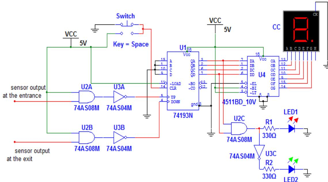
This section consists of up/down counter IC74193, BCD to 7-segment decoder, display driver IC4511 (to drive a common cathode 7-segment display), and three LEDs (red, yellow and green).
