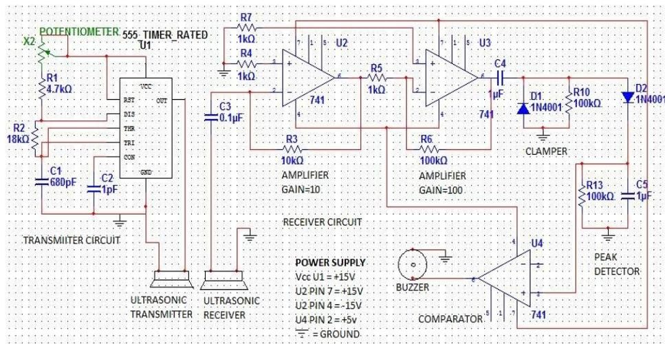
For this particular application, the required components are NE555 (TIMER), Op-amps (741), two 40 kHz ultrasonic transducers (one each for transmitter and receiver), and some discrete components. Ultrasonic generators use piezoelectric materials such as zinc or lead zirconium tartrates or quartz crystal. The material thickness decides the resonant frequency when mounted and excited by electrodes attached on either side of it.
