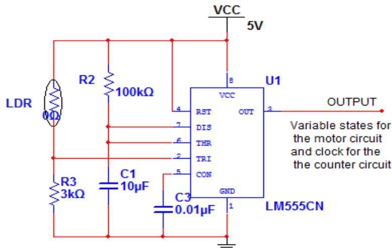
This section senses the movement of objects and transfers that information to the gate control section and counter sections. The output of this section acts as input to the motor driver and assists in gate control mechanism.
