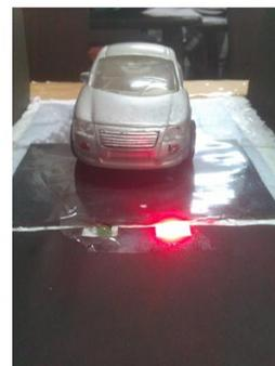
The red LED shows the presence of car being parked. The same signal after inversion is given to the anode of the green LED, which indicates the availability of space for parking.
