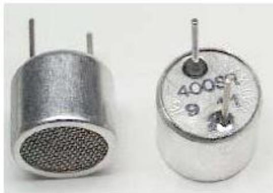
Fig. 1: Ultrasonic transmitter and receiver pair.
