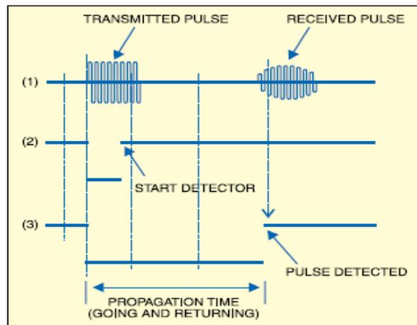
**Fig. 2:** Transmitted and Received Pulses.
