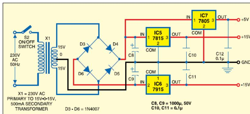
**Fig. 3:** Power Supply Circuit.
