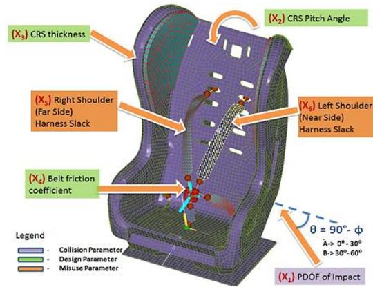
Fig. 6: CRS parameters considered for oblique side impact.
