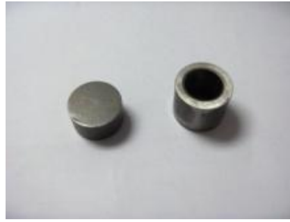
Fig. 16: Work-piece and cup shaped forging produced experimentally.
