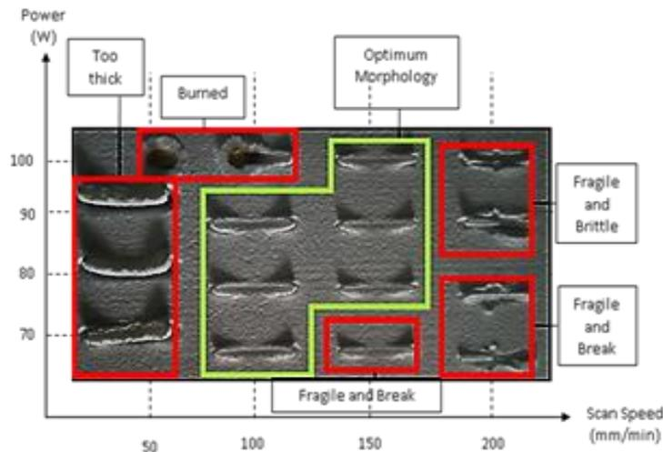
**Fig. 5:** Effect of laser parameters on the surface morphology of single track sample.
