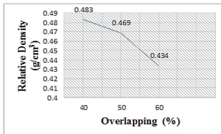
**Fig. 7:** Change of relative density for scan speed of 150mm/min and overlap spacing of multiple track samples.
