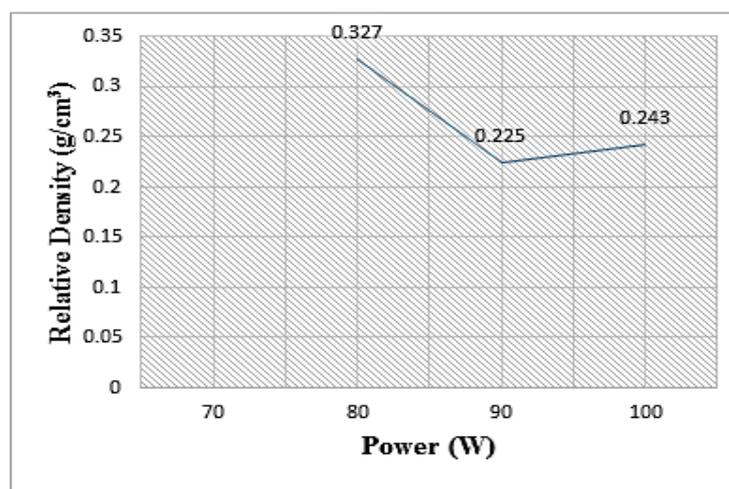
**Fig. 4:** Change of relative density (g/cm<sup>3</sup>) for scan speed 150 mm/min of single track sample.
