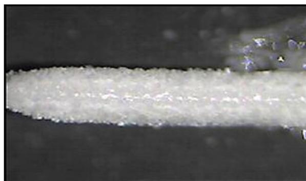
**Fig. 6:** Surface morphology for 150 mm/min scan and 80W laser power of single track sample.
