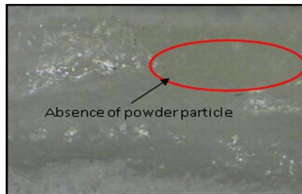
**Fig. 9:** Magnified view of the effect of 130 mm/min scan speed and 60% overlapping percentage on surface morphology showing no presence of unsintered powder particle.
