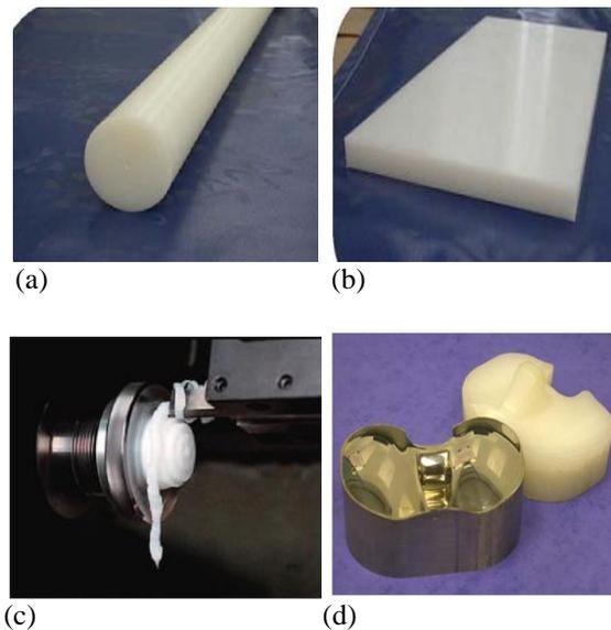
**Fig. 2:** Sample parts produced by (a) ram extrusion, (b) compression mould, (c) machining and (d) direct compression mould
