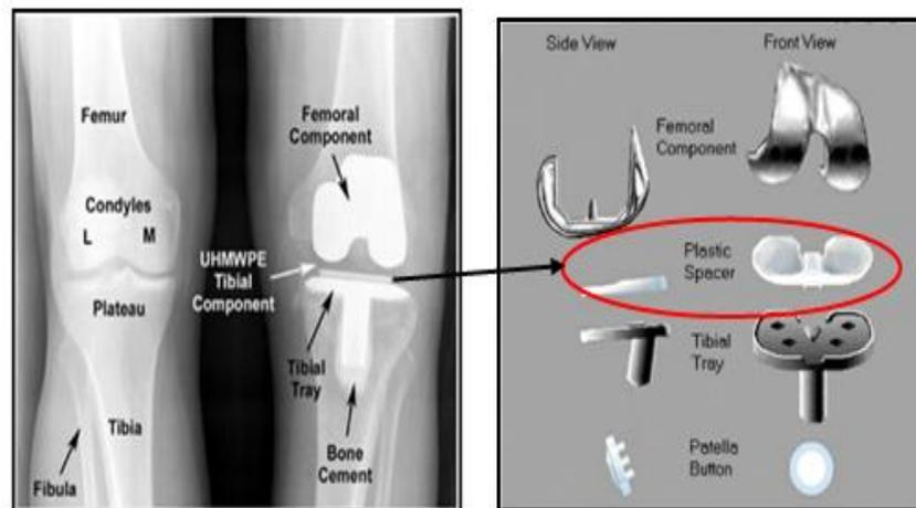
**Fig. 1:** Adaptation of UHMWPE as plastic spacer in Knee Joint Replacement
