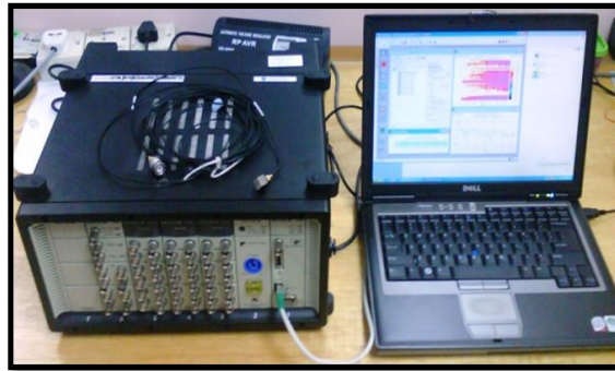
Fig. 1: The Bruel&Kjaer PULSE™ Multi-Analyzer System connect to a computer with MTC™ software and Operational Modal AnalysisPro™ software.
