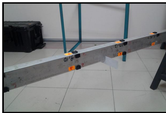
Fig. 2: Aluminum beam and crack position.
