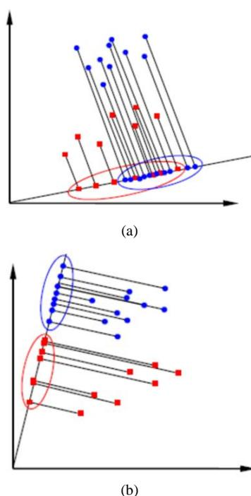
**Fig. 2:** LDA algorithm (a) Data mixed as projected onto a projection line, (b) Data separate as projected onto an optimal projection line.
