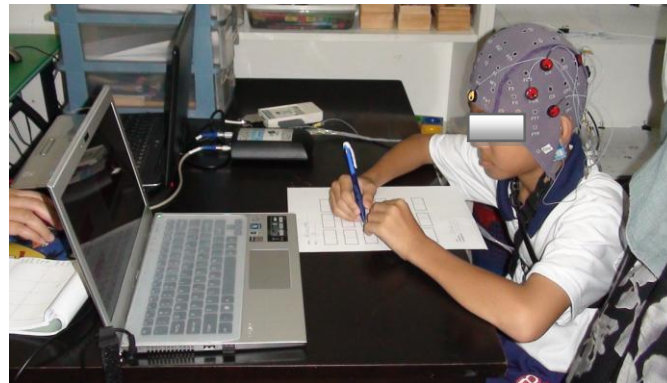
Fig. 3: EEG recording session for a dyslexic child performing the letter writing task.
