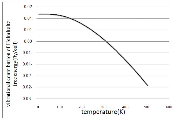
Fig. 5: Vibrational contribution of Helmholtz free energy as a function of temperature in 7/49 a.u. lattice parameter.
