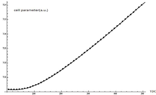
**Fig. 6:** Lattice thermal expansion curve in the quasi-harmonic approximation.
