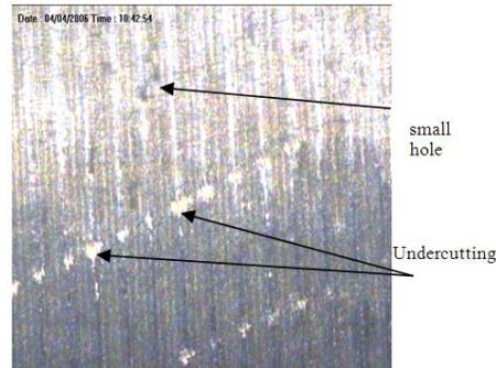
**Fig. 20:** Surface of specimen I.
