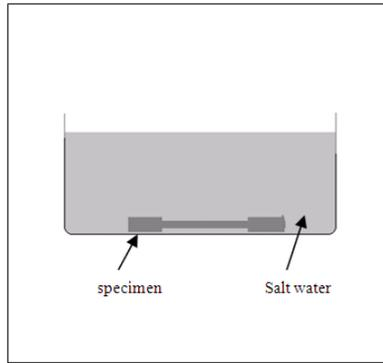
**Fig. 2:** Positioning of specimen immersed in salt water.
