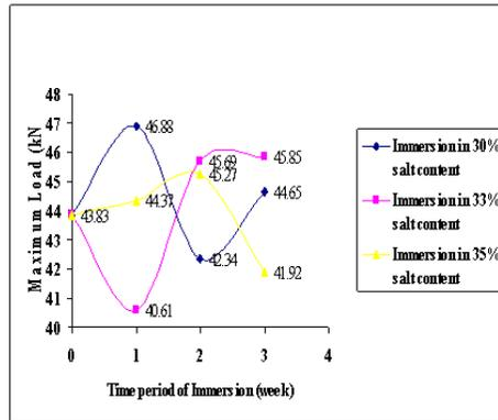
Fig. 10: Graph maximum load versus time period of immersion.
