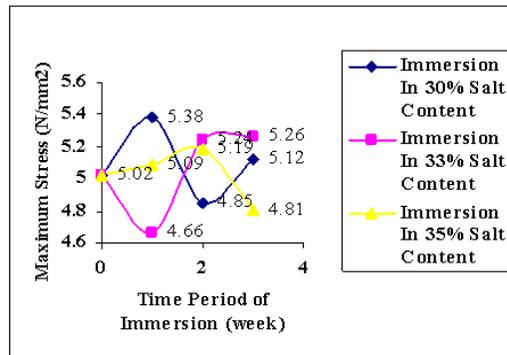
Fig. 11: Graph maximum stress versus time period of immersion.
