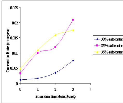
**Fig. 4:** Corrosion rate versus time period of immersion graph.
