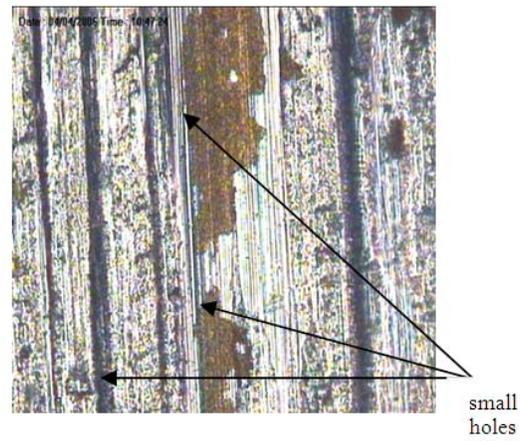
**Fig. 13:** Surface of specimen B.
