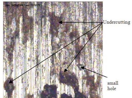
**Fig. 19:** Surface of specimen H.
