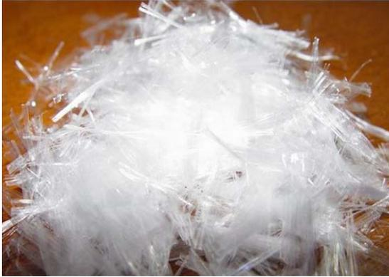
**Fig. 1:** Polypropylene fibre mega mesh
