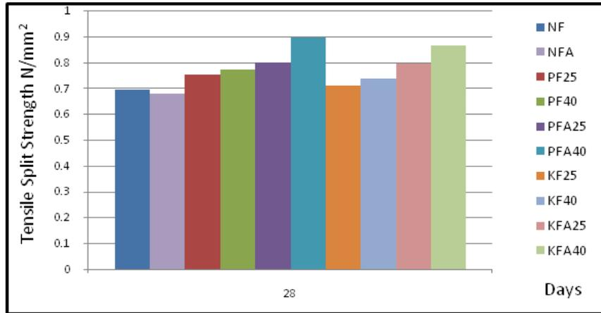
**Fig. 8:** Kenaf and polypropylene fibre concrete tensile splitting strength
