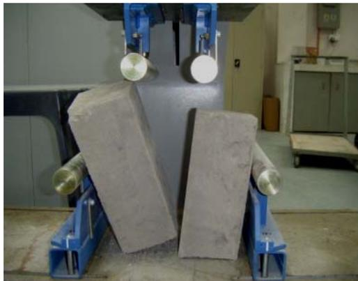
**Fig. 4:** Complete failure of control specimen with the inclusion of fibre
