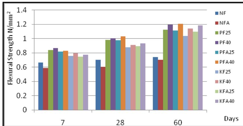
Fig. 7: Kenaf and polypropylene fibre concrete flexural strength
