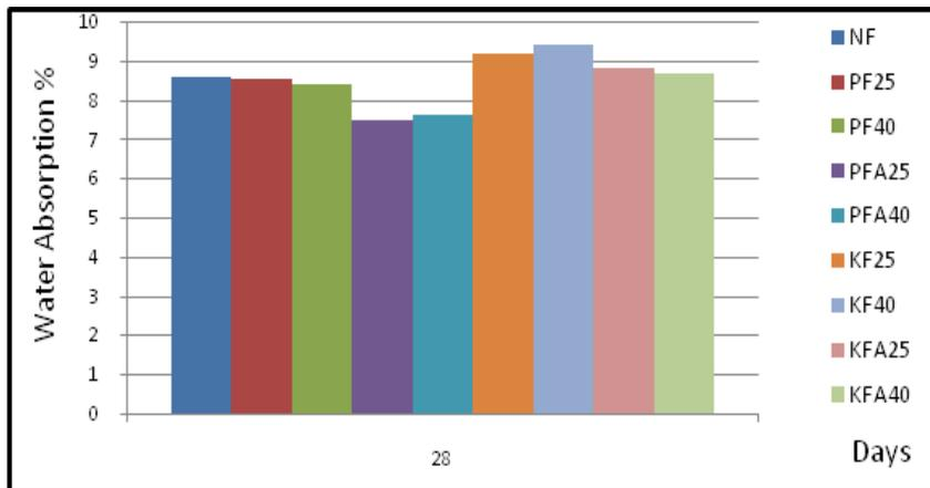
**Fig. 9:** Kenaf and polypropylene fibre concrete water absorption
