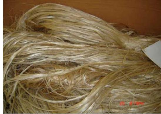
**Fig. 2:** Kenaf fibre (bast)
