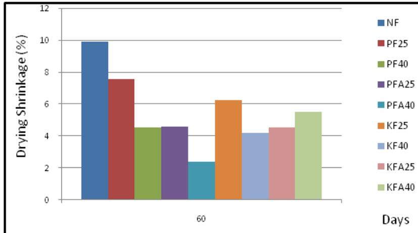
Fig. 10: Percentage of drying shrinkage of kenaf and polypropylene LFC up to 60 days
