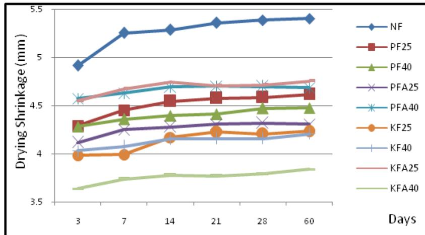
Fig. 11: Drying shrinkage of kenaf and polypropylene LFC by days of test
