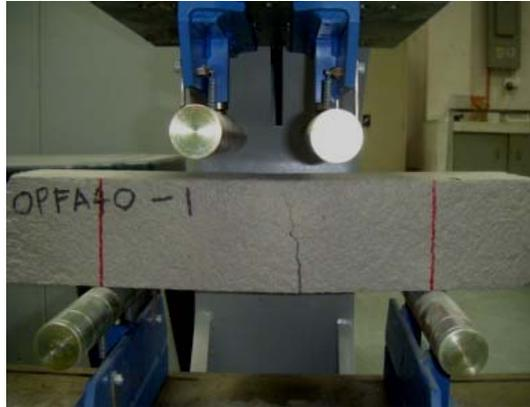
Fig. 5: Progress of 4 point bending test of specimen with fibre inclusion
