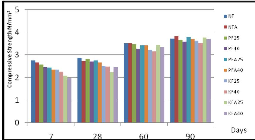
**Fig. 3:** Kenaf and polypropylene fibre concrete compressive strength
