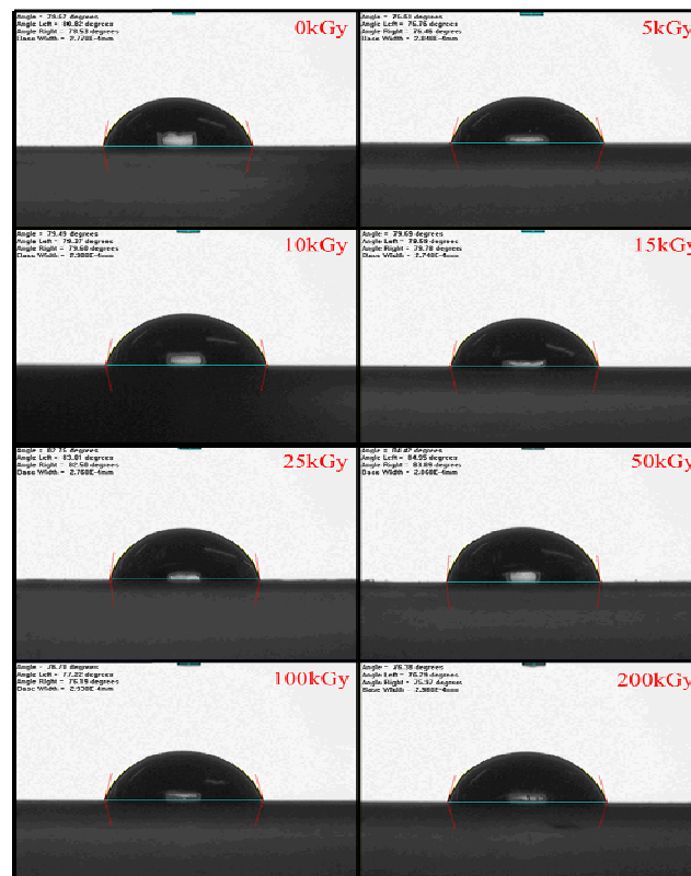
Fig. 8: Images of the droplet on the surface of the non-irradiated and irradiated Pebax tensile specimens
