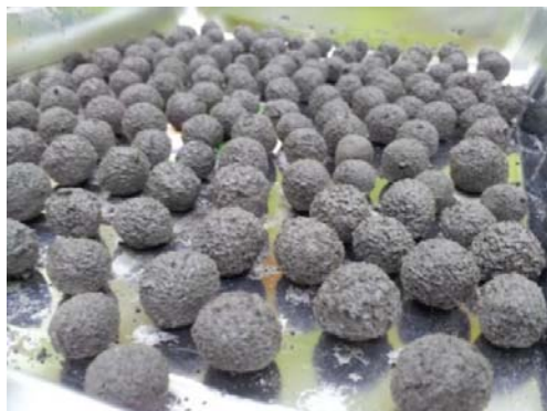
Fig. 1. Pelletized artificial geopolymer aggregate.
