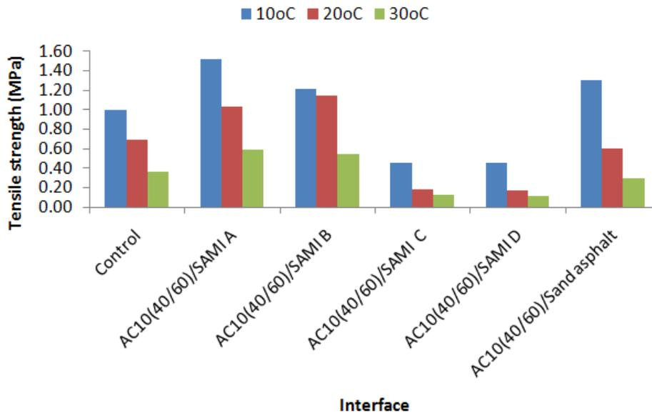
Fig. 3: Pull of test results at 10°C, 20°C, 30°C.
