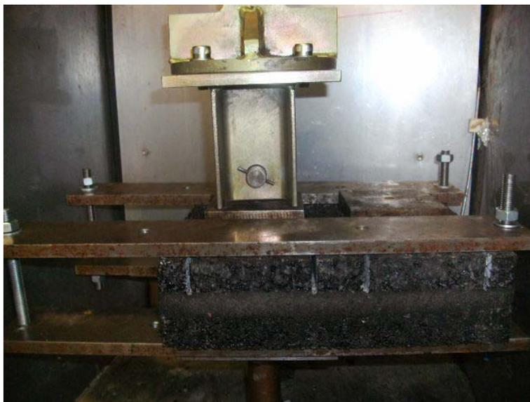
**Fig. 1:** Pull-off test set up.
