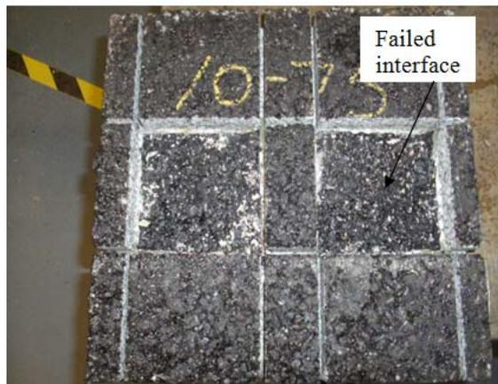
**Fig. 4:** A typical failed interface after test.
