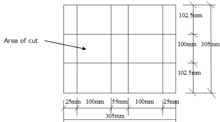
**Fig. 2:** Plan of cuts for the 305 mm × 305 mm slab.
