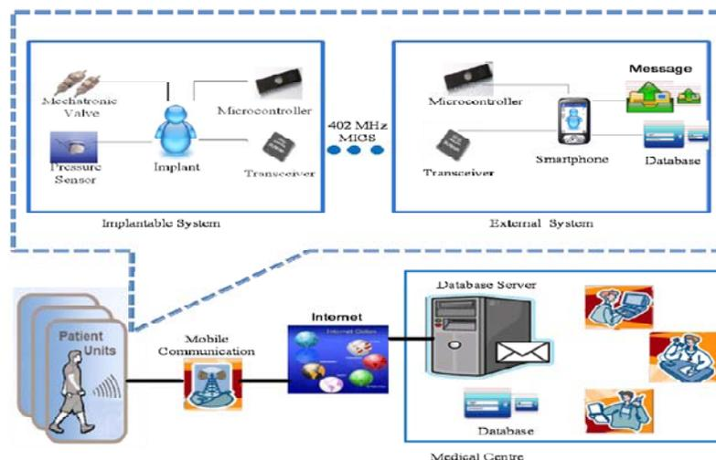
**Fig. 1:** The proposed mechatronic shunting system.
