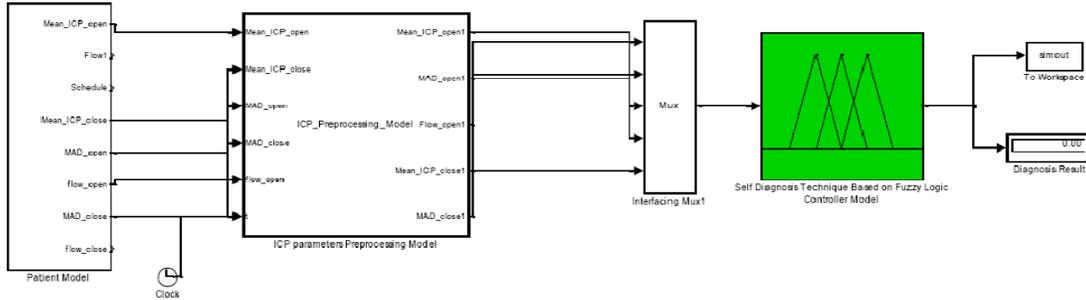
**Fig. 2:** A block diagram of the Simulink set-up for the self diagnosis system.
