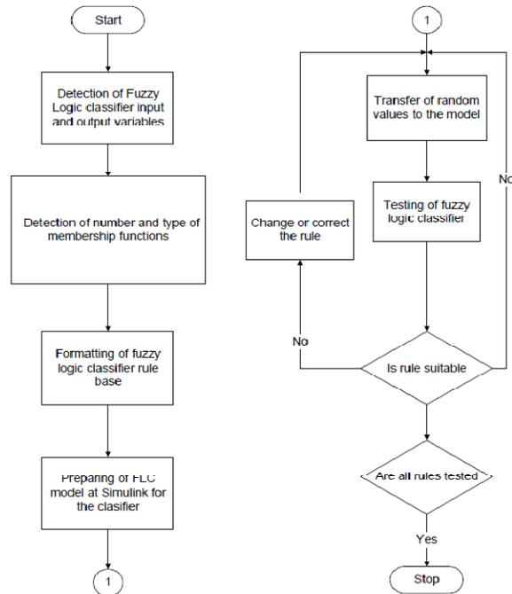
Fig. 6: A flow chart of fuzzy logic classifier design.
