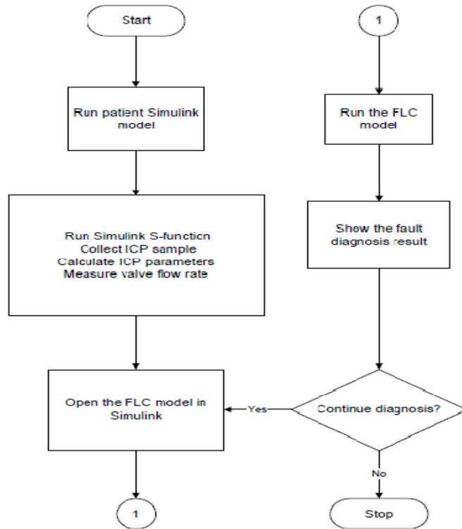
Fig. 5: A flow chart of the fuzzy logic fault diagnosis system.
