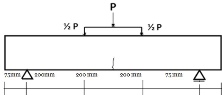
Fig. 3: Arrangement of Bending test
