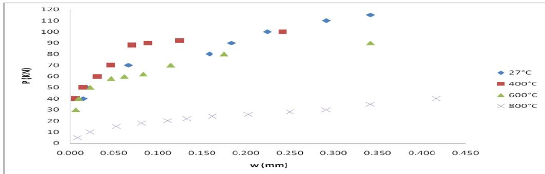
**Fig. 5:** The relation of crack width and loading at temperature variation in 20 mm concrete cover
