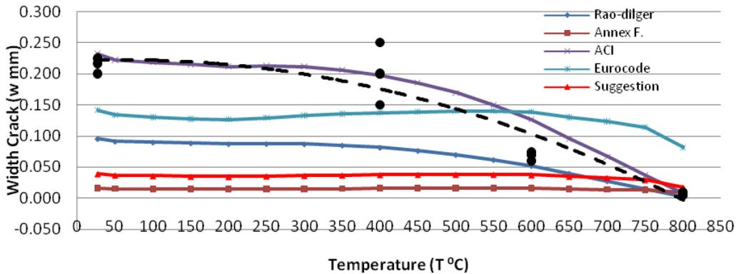
Fig. 9: The relation of crack width and temperature at 25 mm concrete cover in many formula
