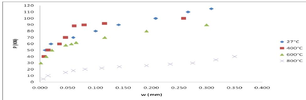
**Fig. 4:** The relation of crack width and loading at temperature variation in 15 mm concrete cover
