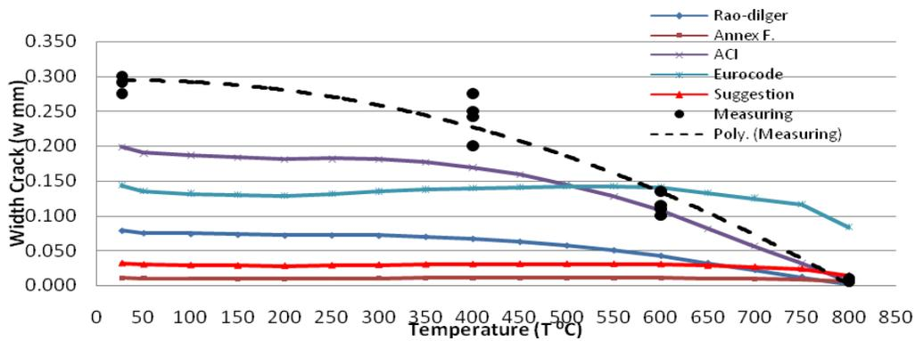
Fig. 8: The relation of crack width and temperature at 20 mm concrete cover in many formula
