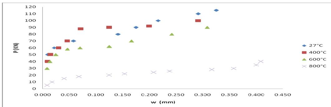
**Fig. 6:** The relation of crack width and loading at temperature variation in 25 mm concrete cover
