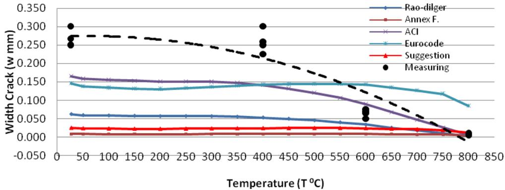
Fig. 7: The relation of crack width and temperature at 15 mm concrete cover in many formula
