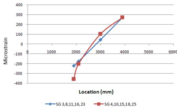
Fig. 14: Shear strains of beam's vertical web due to eccentric loadings.
