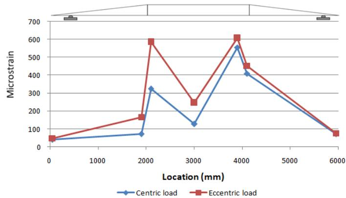
Fig. 12: Axial tensile strains distribution at bottom flange of beam.
