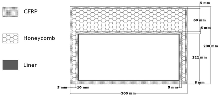
Fig. 2: Cross section of scaled down beam (Centre beam).
