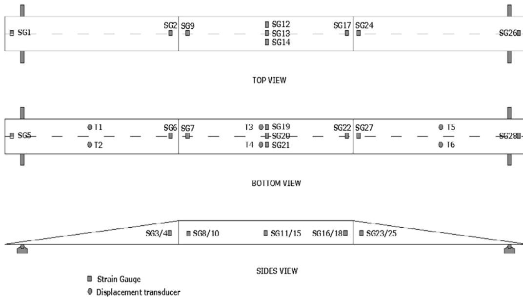
**Fig. 6:** Location of strain gauges and displacement transducer.
