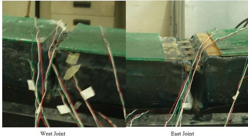
Fig. 10: Detail of west and east joints at failure load.
