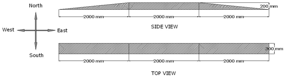
**Fig. 1:** Beam scaled-down prototype dimensions.
