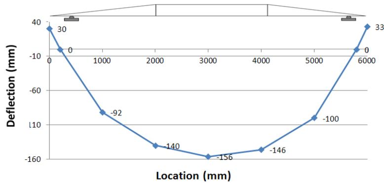
Fig. 8: Maximum vertical displacement distributions on beam due to eccentric load.
