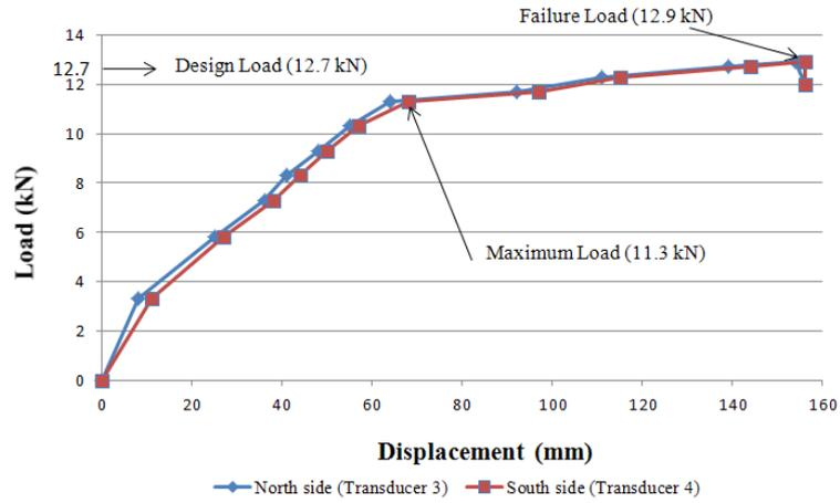
Fig. 7: Load versus displacement on the mid beam for eccentricity load.
