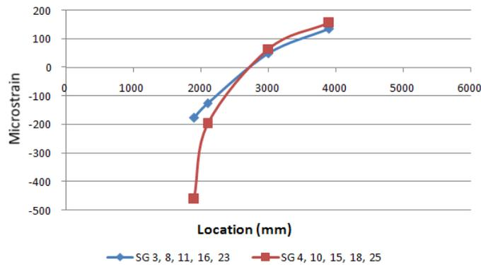
Fig. 13: Shear strains of beam's vertical web due to centric loadings.
