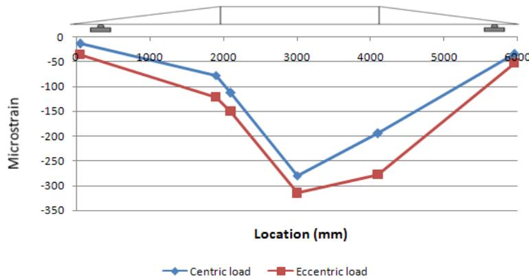
Fig. 11: Axial compressive strains distribution at top flange of beam.
