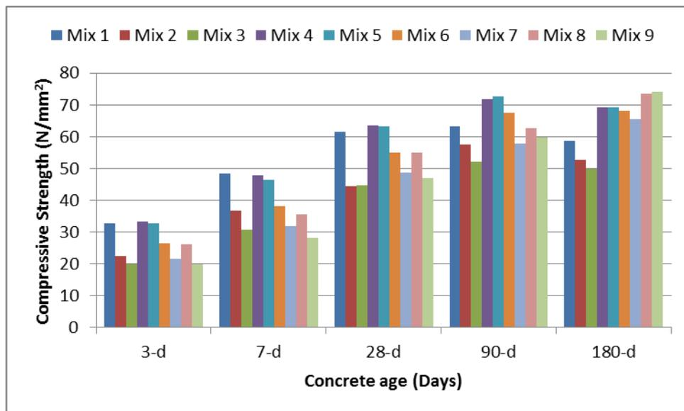
**Fig. 1:** Compressive strength of the studied concretes.
