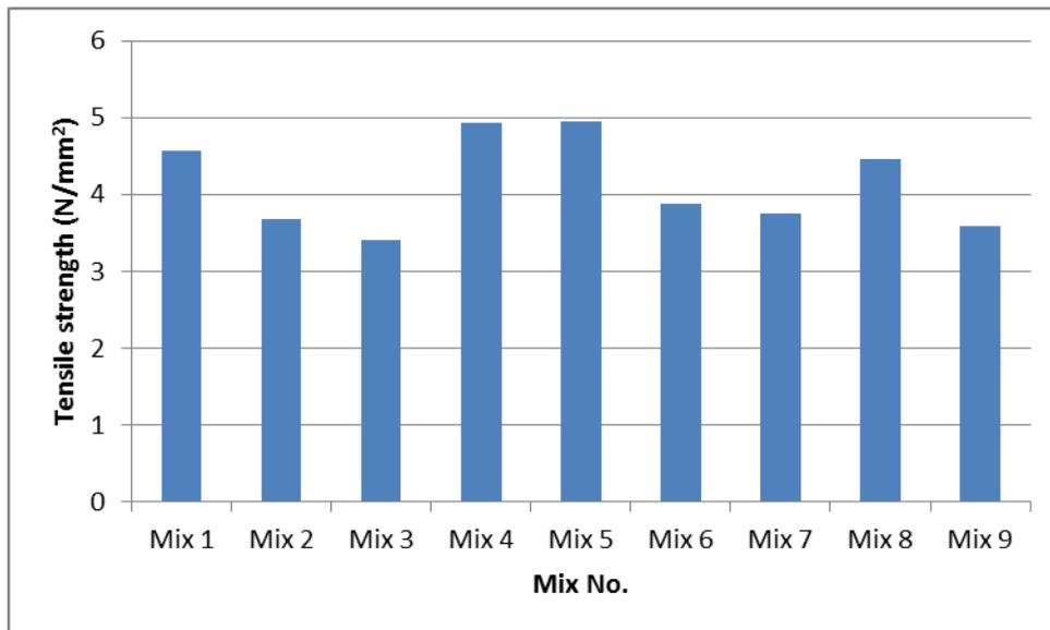
**Fig. 3:** Tensile strength of the studied concretes.
