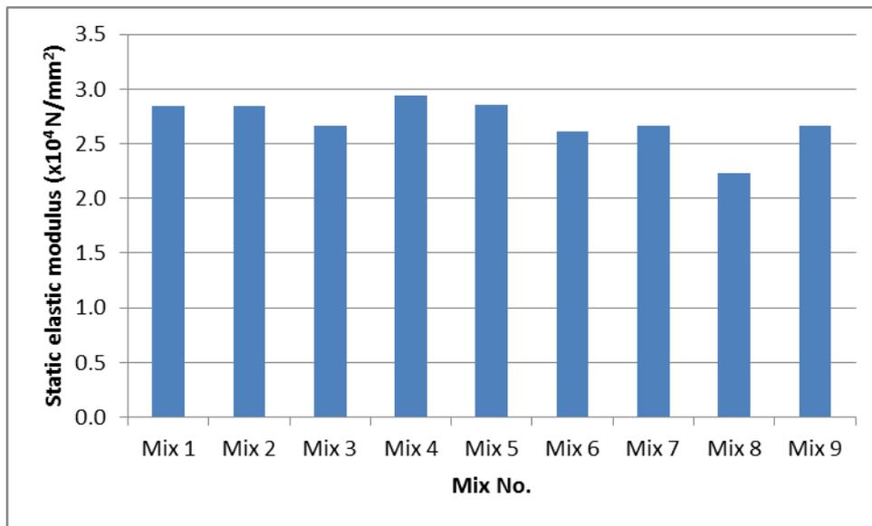
**Fig. 5:** Static elastic modulus of the studied concretes.
