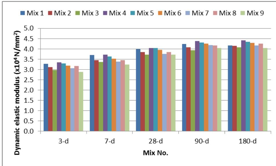
**Fig. 4:** Dynamic elastic modulus of concretes.
