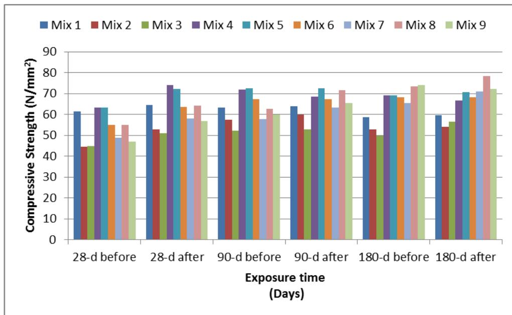
**Fig. 6:** Compressive strength of tested concrete before and after exposure to sodium sulphate.
