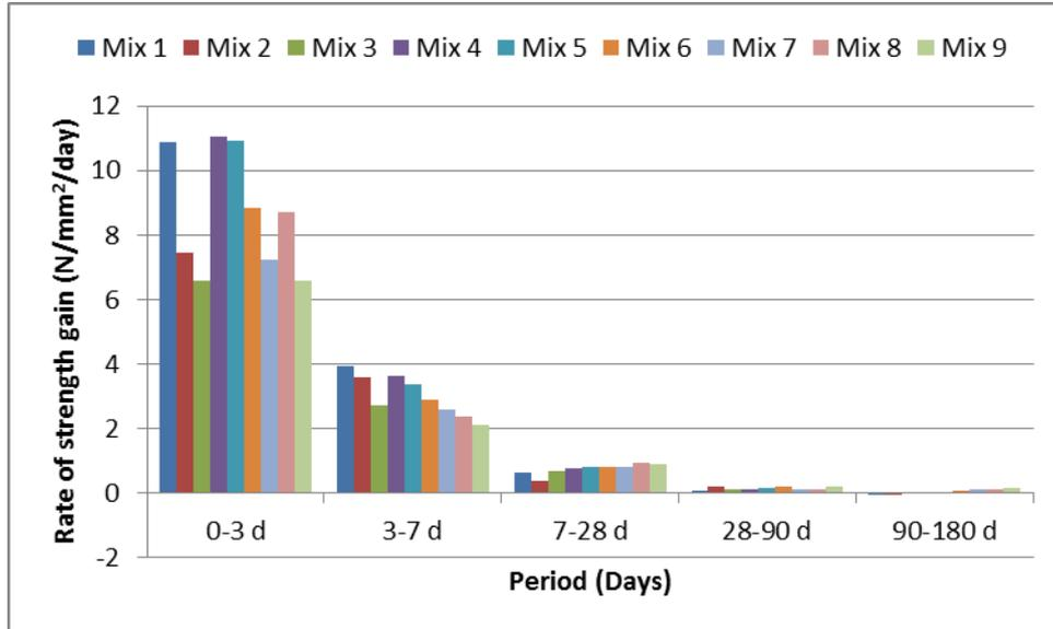
**Fig. 2:** Rate of compressive strength development.
