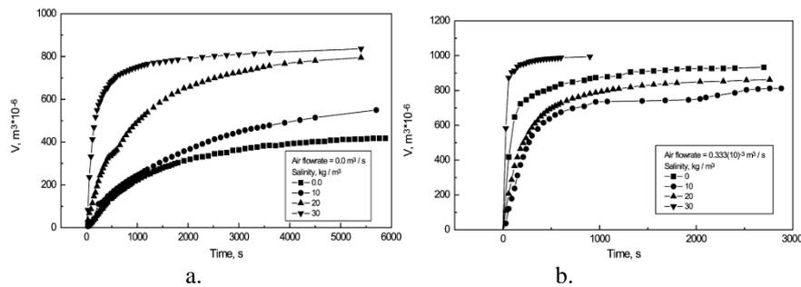
**Fig. 2:** The rate of oil spill clean up using vaccum technique (Mazindouh and Omar, 2003):
