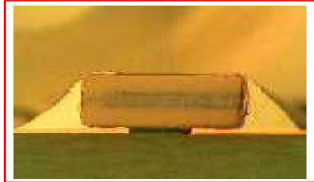
**Fig. 1:** A Typical 0805 Resistor with Solder Joint.
