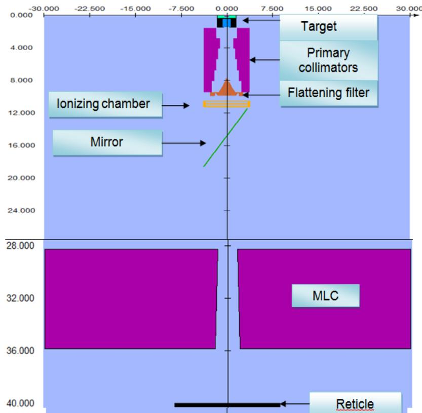
**Fig. 1:** Simulated linear accelerator head (xy view).
