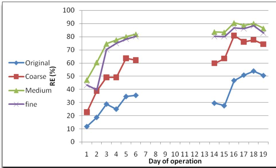
**Fig. 11:** P Removal efficiency at the middle samples for the applied forms
