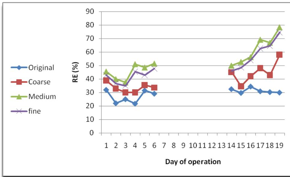
**Fig. 7:** TSS Removal efficiency at the effluent samples for the applied forms
