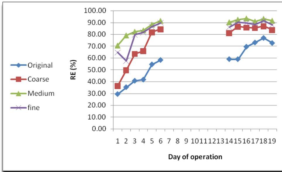
**Fig. 12:** P Removal efficiency at the effluent samples for the applied forms
