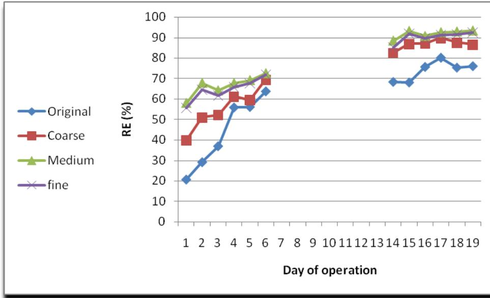
**Fig. 10:** N Removal efficiency at the effluent samples for the applied forms
