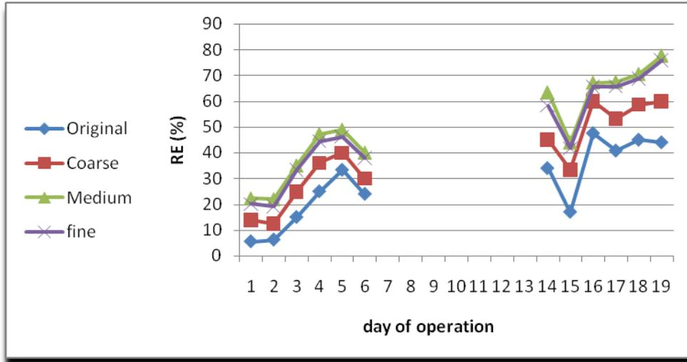
**Fig. 8:** COD Removal efficiency at the effluent samples for the applied forms
