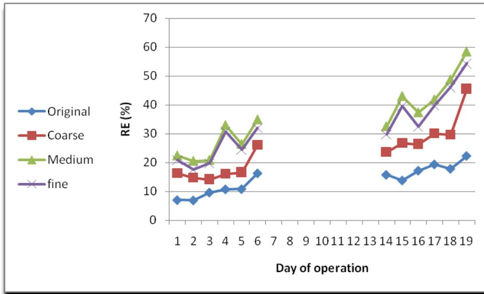
**Fig. 4:** BOD Removal efficiency at the middle samples for the applied forms
