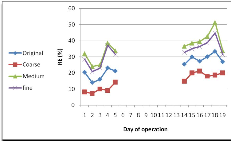
**Fig. 6:** TSS Removal efficiency at the middle samples for the applied forms
