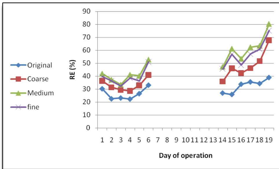
**Fig. 5:** BOD Removal efficiency at the effluent samples for the applied forms
