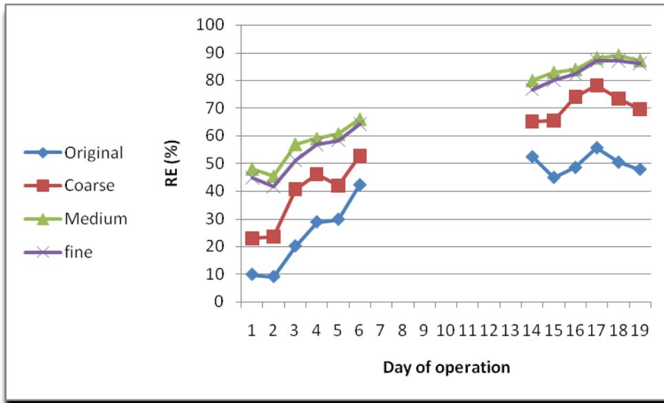
**Fig. 9:** N Removal efficiency at the middle samples for the applied forms
