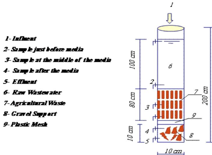
**Fig. 3:** Schematic Diagram of Column Reactor Showing Samples Different Locations
