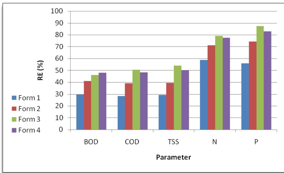
**Fig. 13:** The Average Results at the effluent samples for the applied forms
