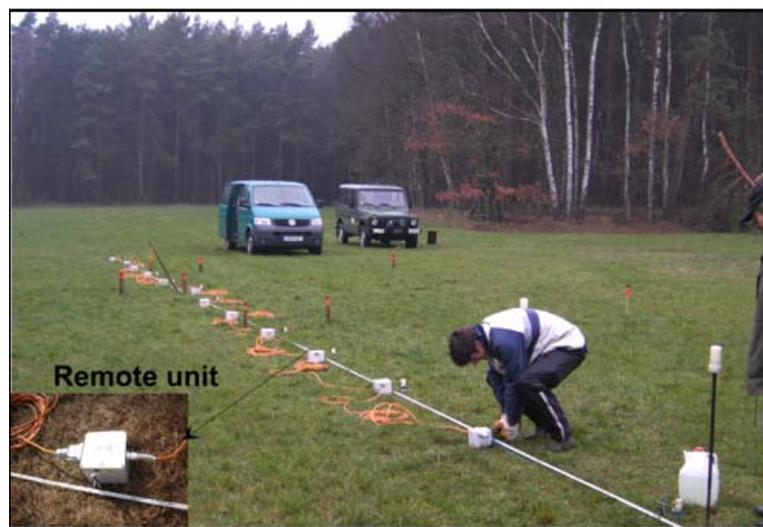
**Fig. 2:** The multichannel SIP equipment by Radic Research (Radic 2004) in operation at a Schillerslage test site in North Germany.
