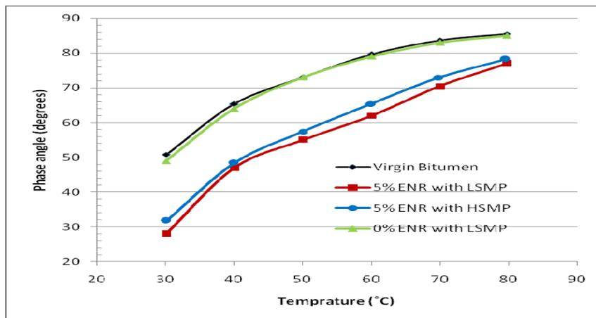
Fig. 6: Isochronal plot of phase angle for long term aged binders.
