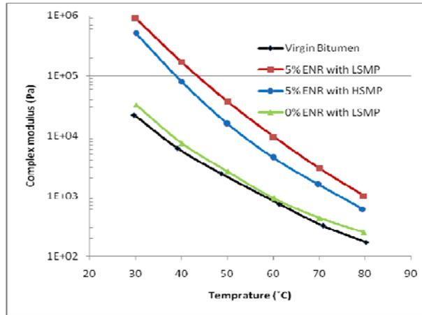
**Fig. 1:** Isochronal plot of complex modulus for unaged binders.
