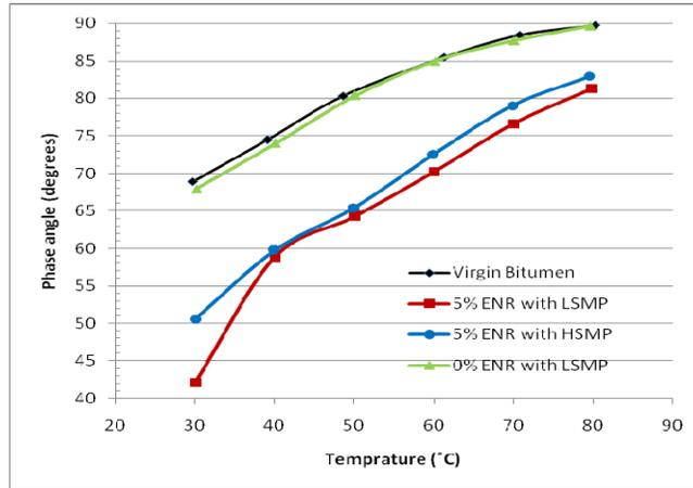
Fig. 4: Isochronal plot of phase angle for unaged binders.
