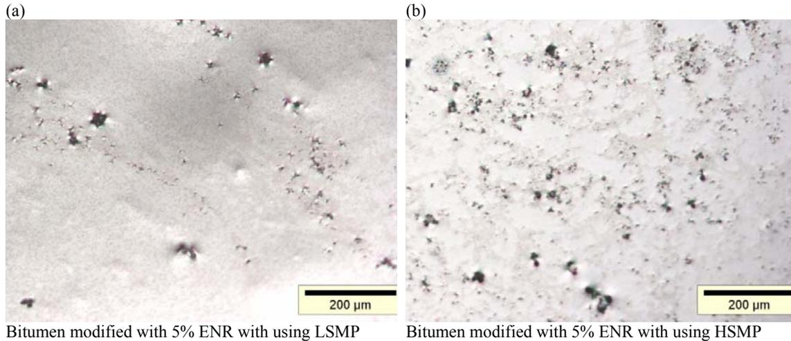
**Fig. 7:** Fluorescent images of ENR modified Bitumen.
