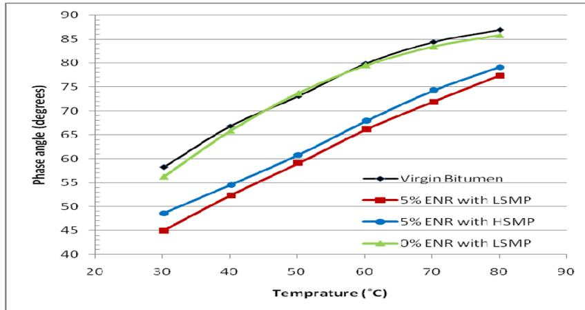
Fig. 5: Isochronal plot of phase angle for short aged binders.
