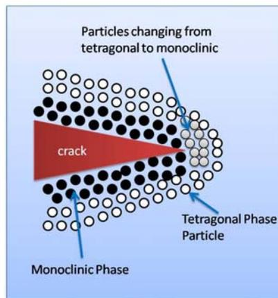
**Fig. 2:** Transformation toughening process of zirconia.
