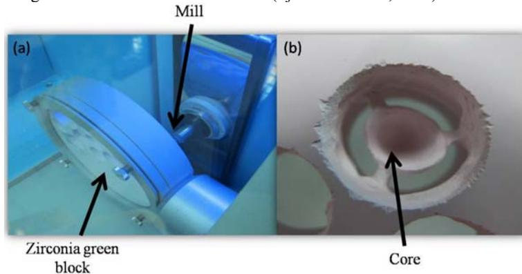
**Fig. 1:** Represent (a) milling process of zirconia Cercon; (b) core of zirconia Cercon.
