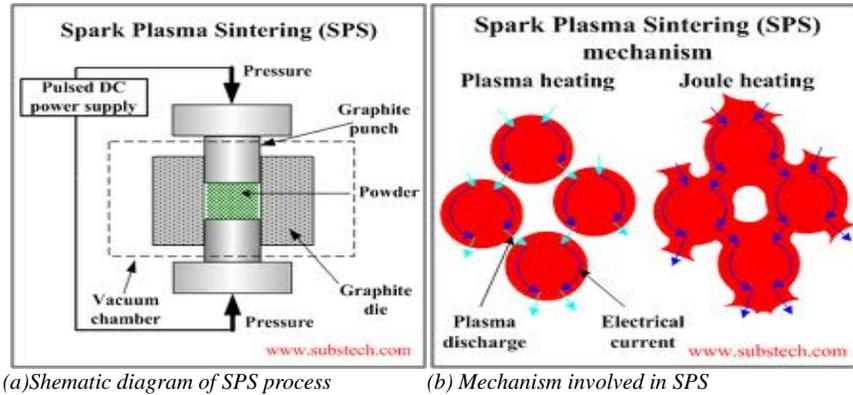
Fig. 5: Spark plasma sintering process (German R.M)
