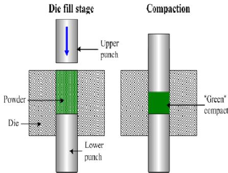
**Fig. 4:** Compaction process (German R.M)
