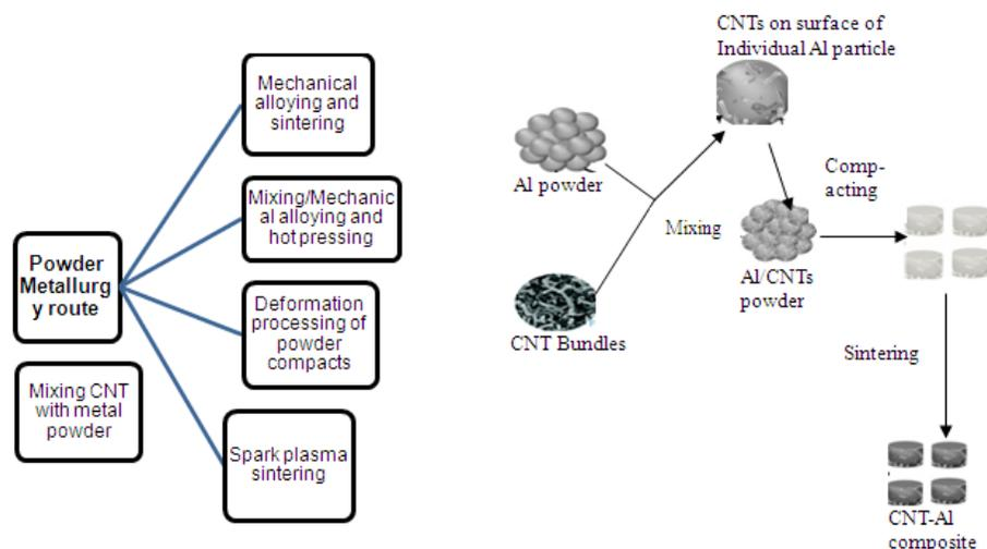
**Fig. 1:** Sub divisions of powder metallurgy route Fig. 2 PM route for Carbon nanotube aluminium nano-composite.
