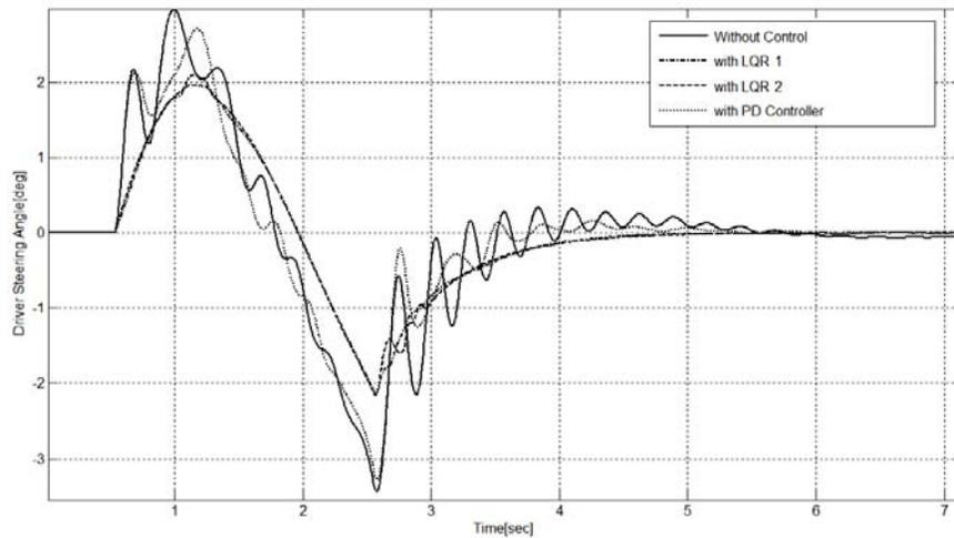
Fig. 9: The driver steering angles in four cases.
