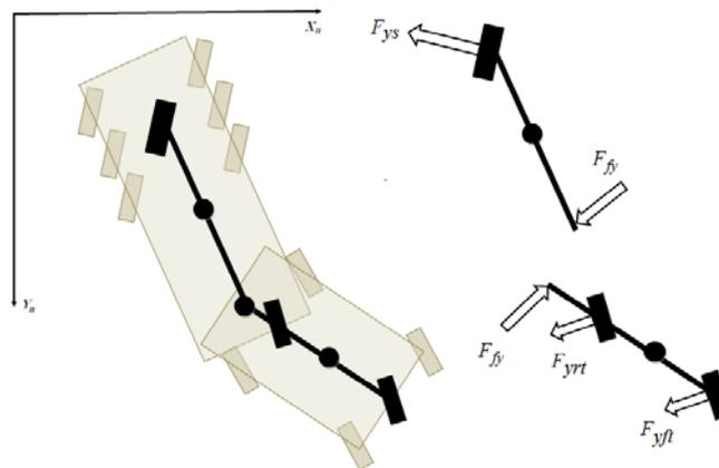
**Fig. 2:** Linear model of the articulated vehicle.
