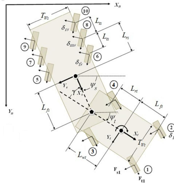
**Fig. 1:** Fourteen degrees of freedom articulated vehicle model.
