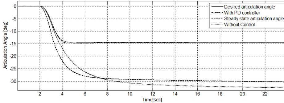
**Fig. 12:** Articulation angle response in low speed turning manoeuvre.
