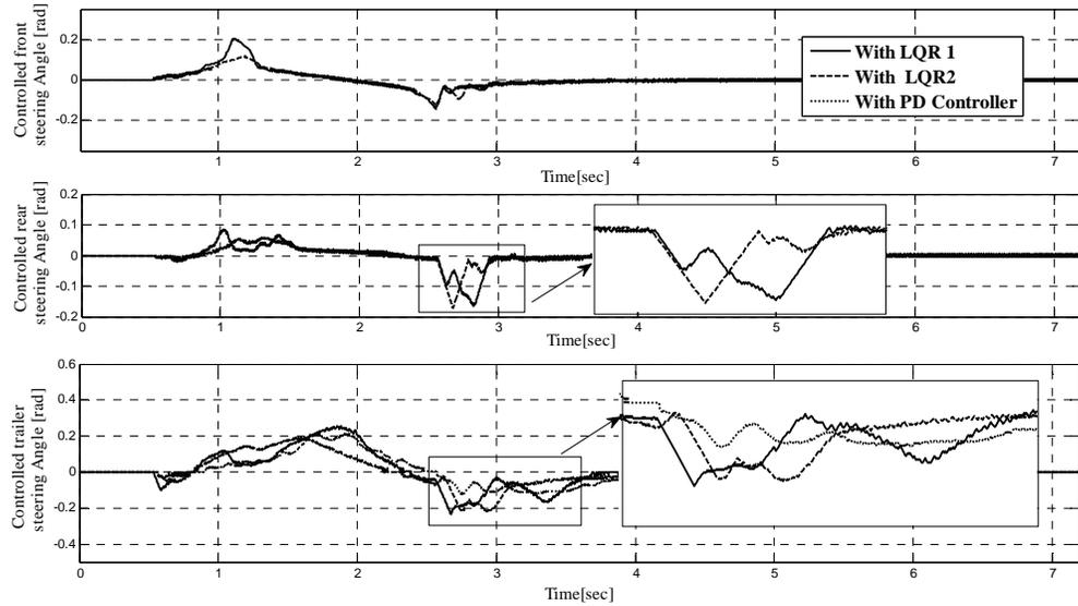
**Fig. 10:** The controlled steering angles of the articulated vehicle axles.
