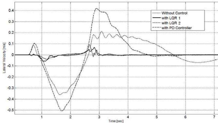
**Fig. 6:** Tractor lateral velocity responses in lane change maneuver.
