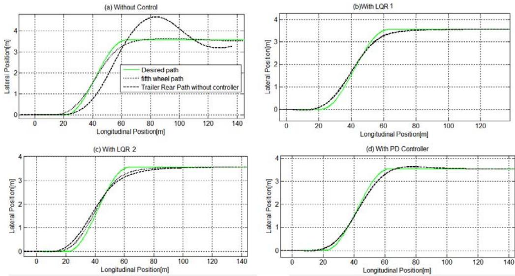
Fig. 8: The vehicle path in the four cases.
