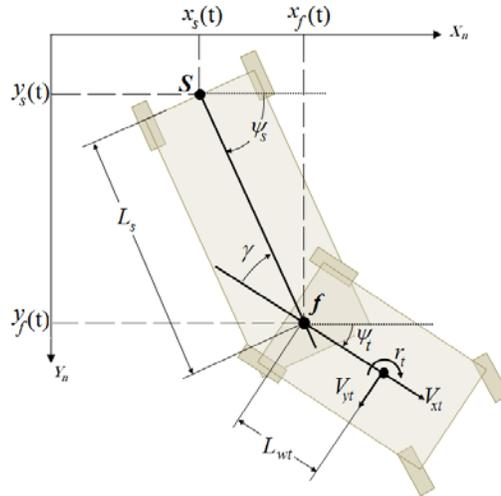
**Fig. 3:** Schematic of the planar motion of the articulated vehicle.
