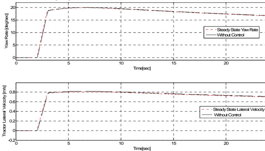
**Fig. 14:** Yaw rate and lateral velocity responses in low speed turning manoeuvre.
