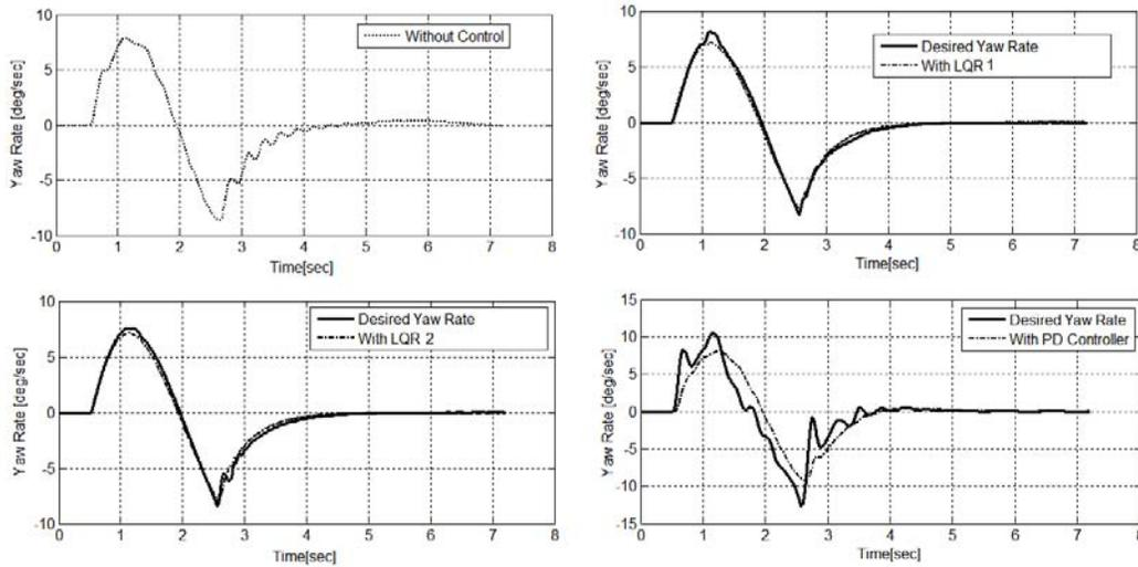
**Fig. 5:** Tractor yaw rate responses in lane change maneuver.
