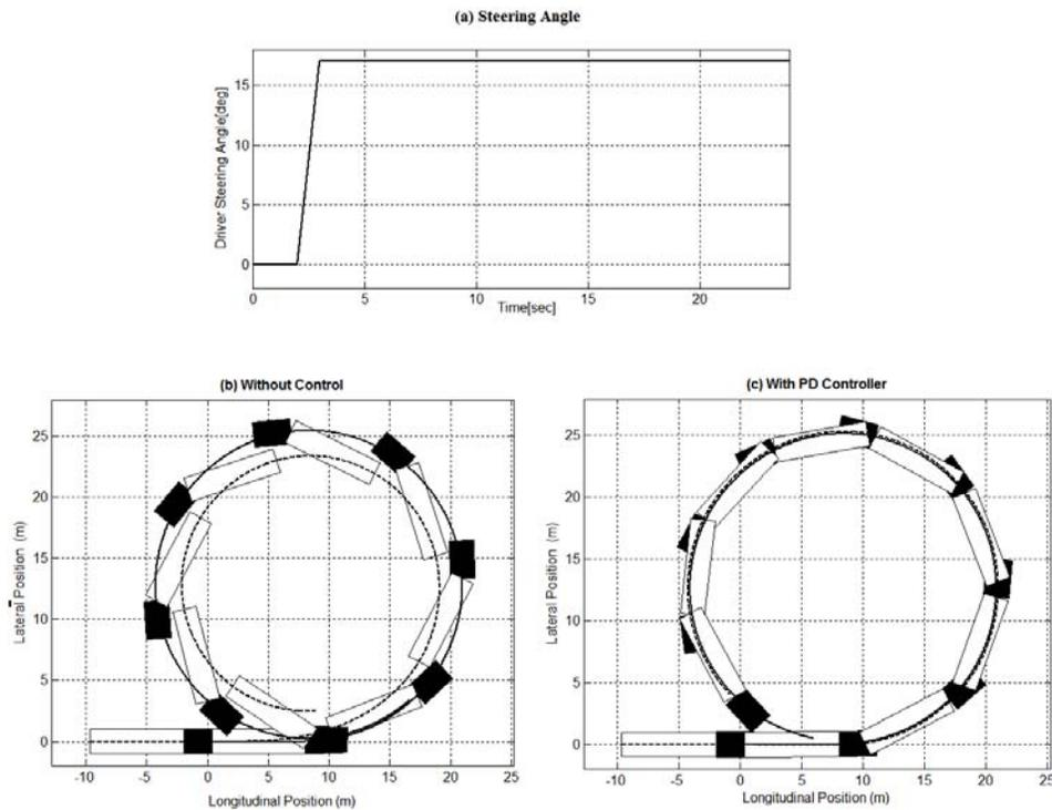
**Fig. 11:** (a) Steering angle in low speed turning manoeuvre, (b) Paths of the vehicle without control, (C) Paths of the vehicle with proposed method
