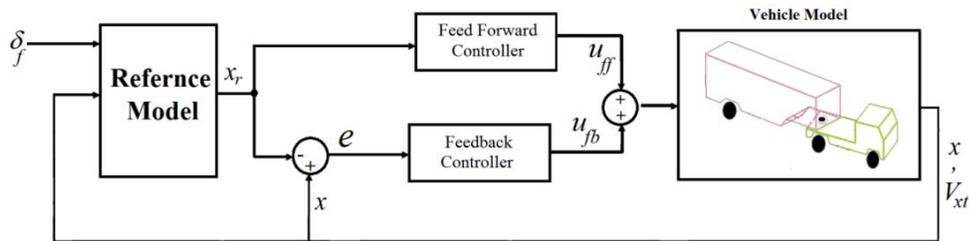
**Fig. 4:** Block diagram of the control system.
