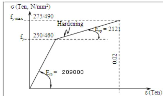
**Fig. 4:** Tensile behavior of steel reinforcement bar.
