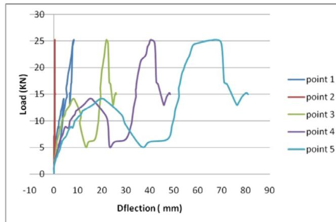
**Fig. 9:** Load-displacement curves of specimen 3.
