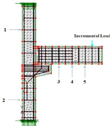
In this case,  $P$  is the incremental point load applied at the beam end, and  $\delta$  is the corresponding deflection under the incremental applied load. Figure 6 shows the various important points that involved in the calculation of displacement.
