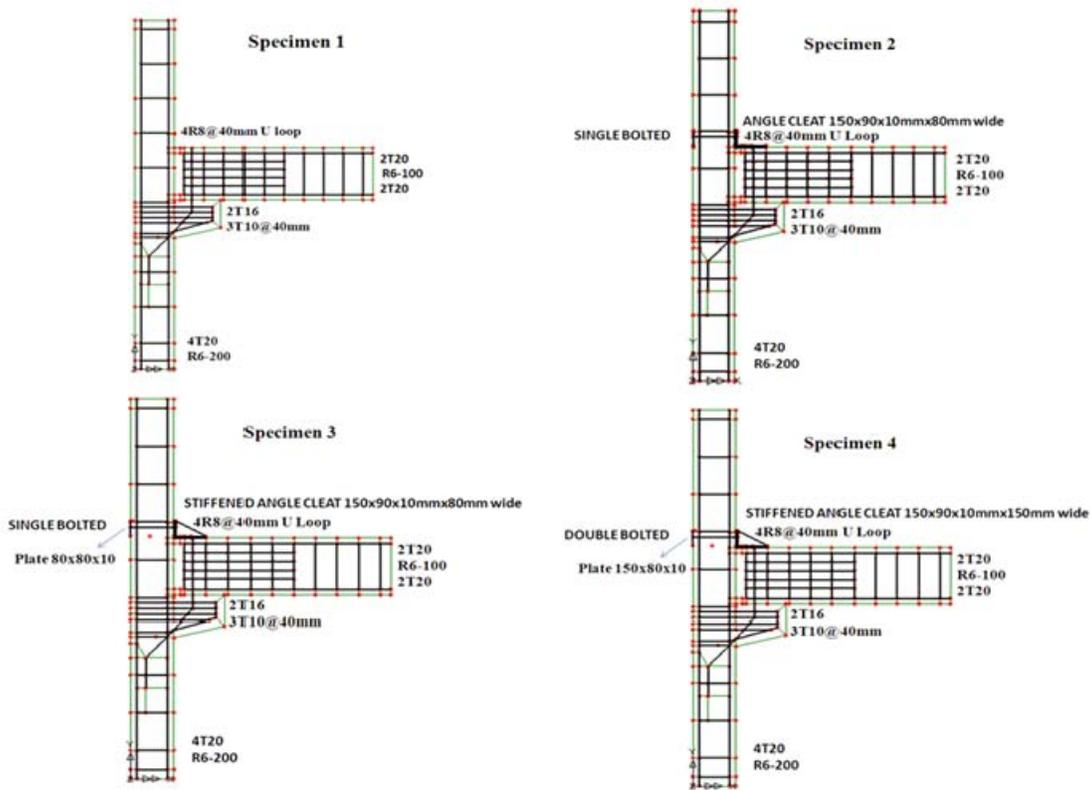
Fig. 1: Geometry of the specimens in LUSAS modeler.
