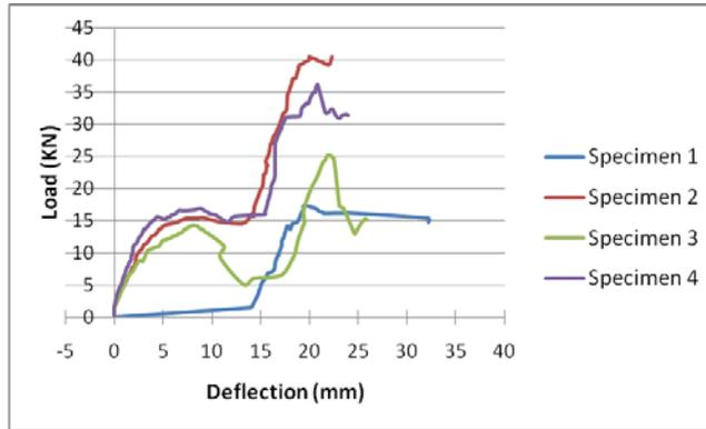
**Fig. 13:** Load-displacement curves at Point 3.
