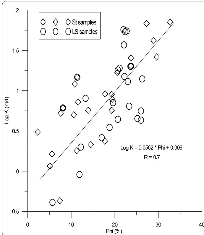
**Fig. 14:** The relationship between Log K and Phi for the all studied samples, R35 (0.5:2)
