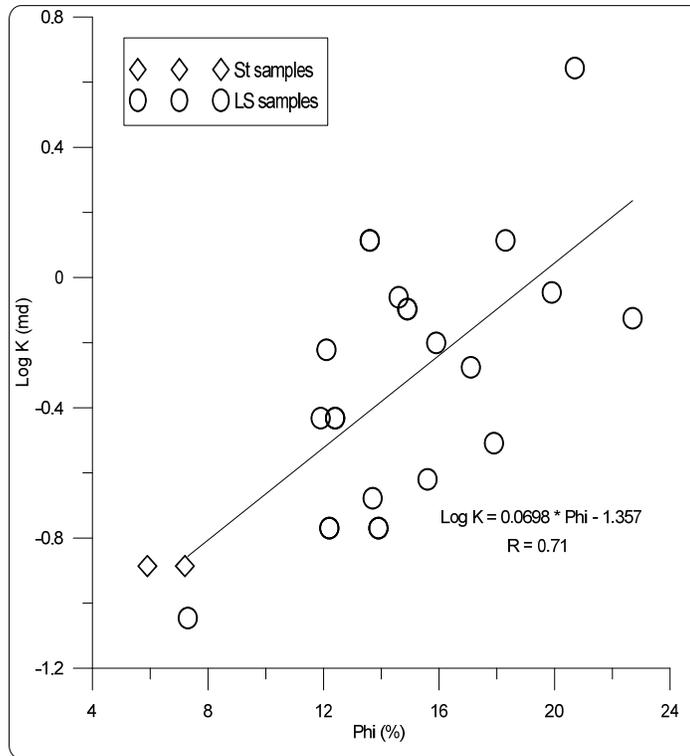
**Fig. 13:** The relationship between Log K and Phi for the all studied samples, R35 (0.1:0.5)
