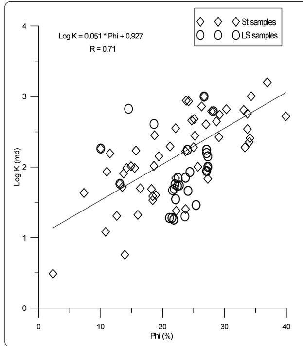
Fig. 15: The relationship between Log K and Phi for the all studied samples, R35 (2:10)
