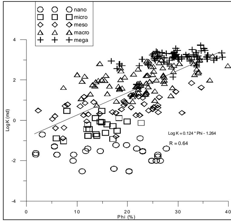
Fig. 11: The relationship between Log K and Phi for the all studied samples.
