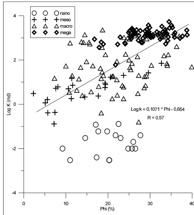
**Fig. 1:** The relationship between Log K and Phi for the all studied sandstons sampies.
