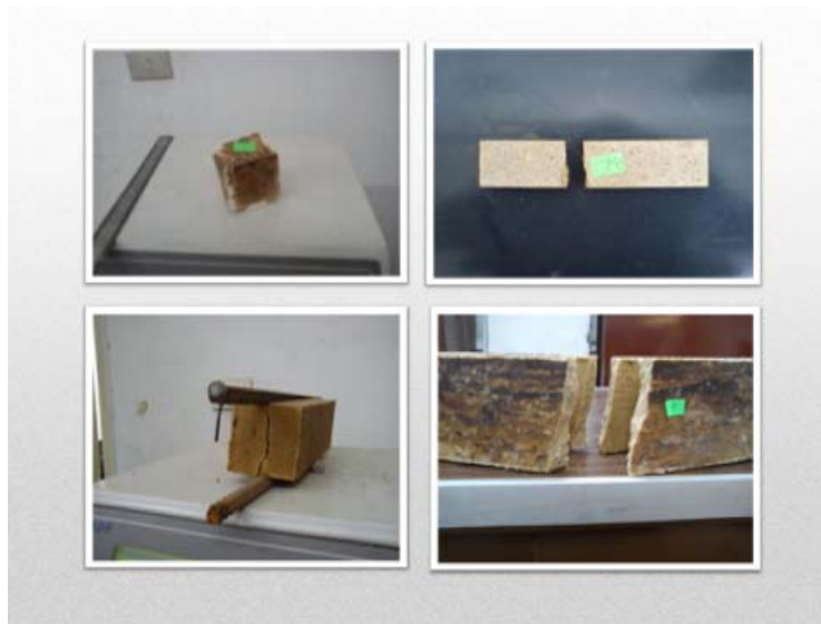
Photo 2: Modes of failure of tested specimens.
