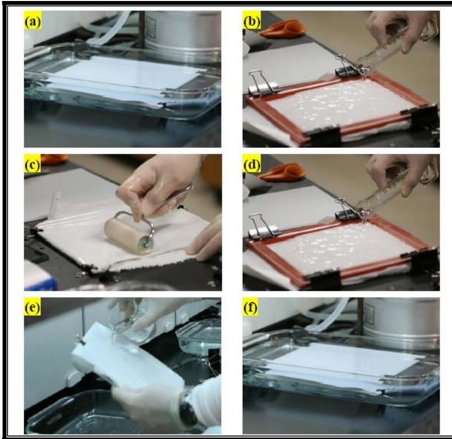
**Fig. 2:** Protocol to prepare polyamide TFC membranes, Xie *et al.*, 2012.
