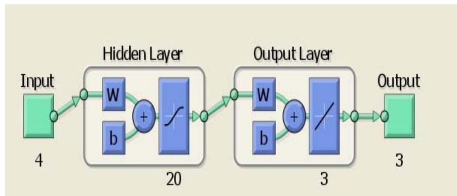
**Fig. 3:** Neural Network Structures with the input, output and hidden neurons
