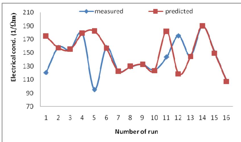
**Fig. 6:** Predicted electrical conductivity of GCE with their corresponding targets at different data points
