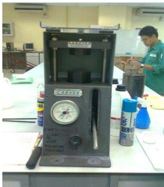
**Fig. 2:** The carver press used for compaction
