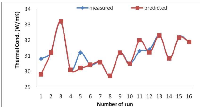
**Fig. 5:** Predicted thermal conductivity of GCE with their corresponding targets at different data points
