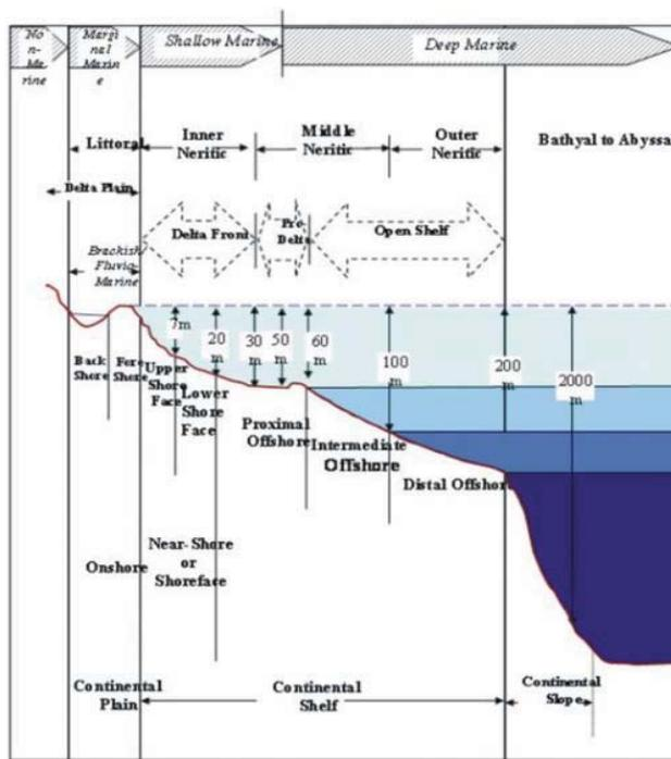
**Fig. 14:** Depositional Environments and Bathymetric Ranges (after, Alle, 1965; 1970)
