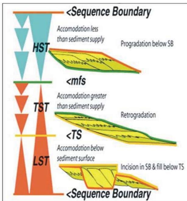
**Fig. 15:** Sequence Stratigraphic Model for the Interpretation of Systems Tracts and Accompanying Key Stratigraphic Surfaces (after, Van Wagoner *et al.*, 1988)
