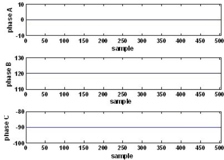
**Fig. 9:** Phase waveforms for an unbalanced signal.
