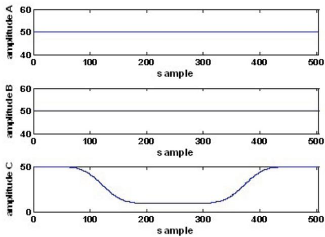
Fig. 13: Amplitude curves for sag type B.
