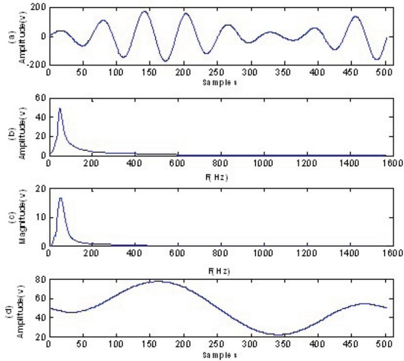
Fig. 7: Voltage flicker and extracted curves
