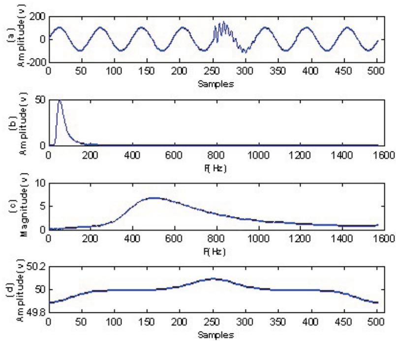
Fig. 5: Oscillatory transient and extracted curves.
