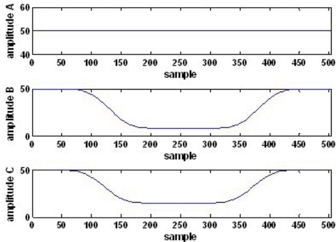
Fig. 19: Amplitude curves for sag type E.
