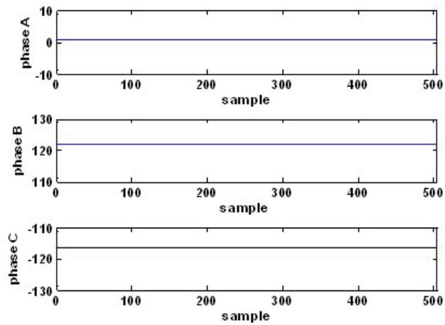
Fig. 12: Phase curves for sag type B.
