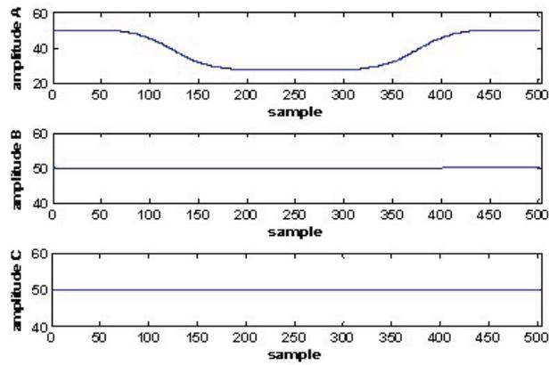
Fig. 17: Amplitude curves for sag type D.
