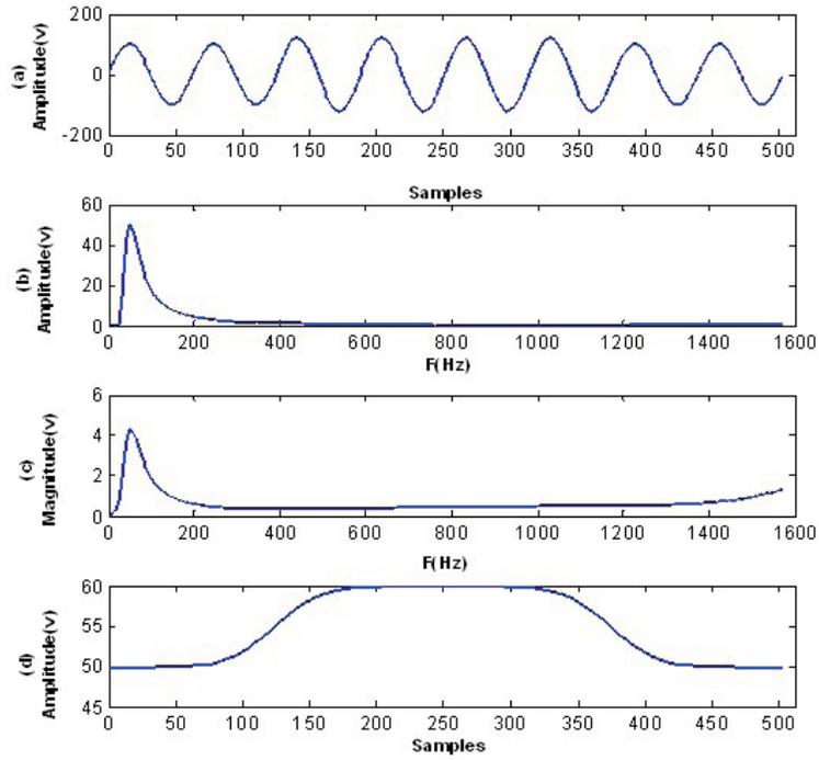
Fig. 3: Voltage swell and extracted curves
