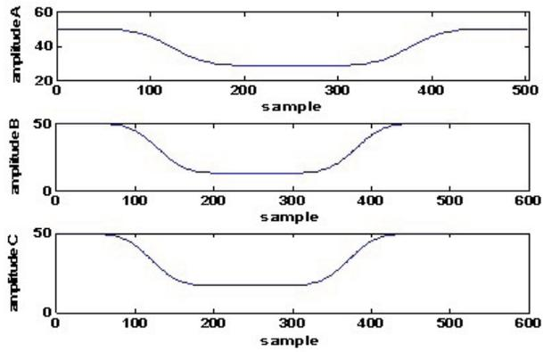
Fig. 11: Amplitude curves for sag type A.
