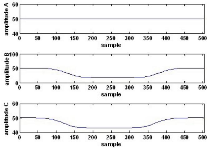
Fig. 15: Amplitude curves for sag type C.
