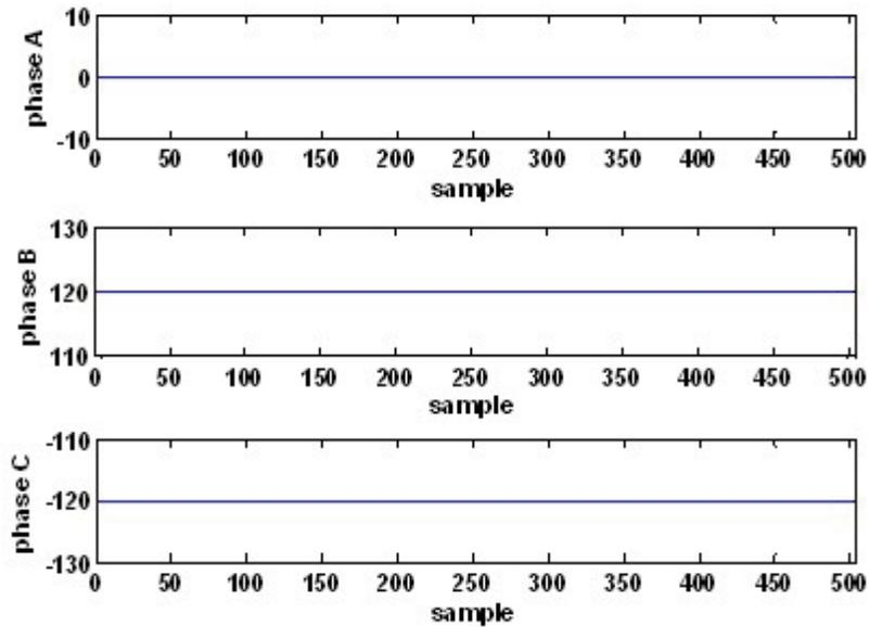
Fig. 8: Phase waveforms for a balanced signal.
