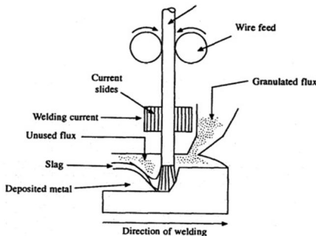
**Fig. 1:** A schematic of SAW process (Kumanan and *et al.*, 2007)
