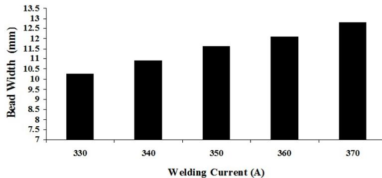
**Fig. 4:** Bead Width vs. welding current diagram for V=26 V & S=52 cm/min
