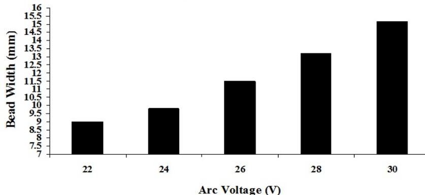
**Fig. 5:** Bead width vs. arc voltage diagram for I=350A & S=52 cm/min
