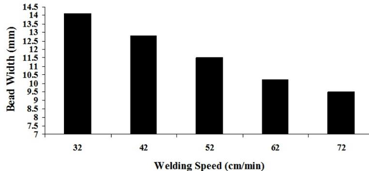
**Fig. 6:** Bead width vs. welding speed diagram for I=350A & V=26 V
