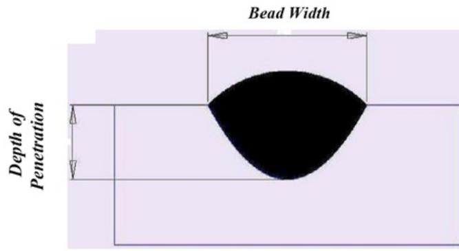
**Fig. 2:** A schematic illustration of bead geometry
