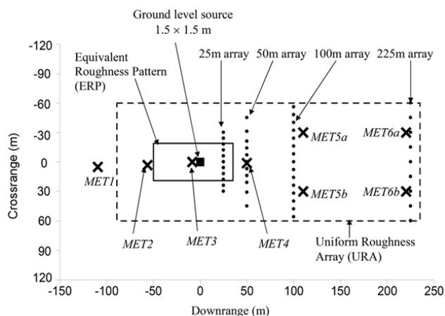
**Fig. 1:** Plot plan of the Kit Fox dispersion grid including meteorological towers, concentration monitoring arcs, gas source, Equivalent Roughness Pattern (ERP), and Uniform Roughness Array (URA) (Hanna and *et al.* (1999).
