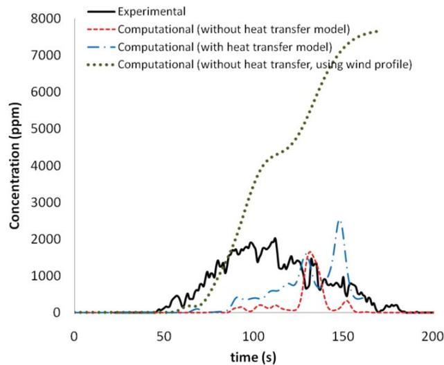
**Fig. 13:** Comparison of experimental and computational results in Kit Fox experiment (trial 3-7) on arc two, at height 0.5m.
