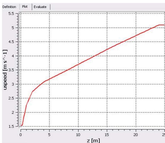
**Fig. 9:** u component of wind speed from 10 to 20 second after gas release in EPA tower location that included to the simulation
