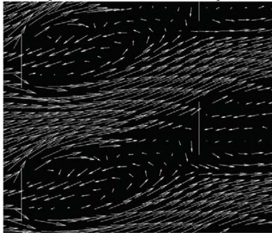
Fig. 5: Flow vectors rear of obstacles on the horizontal plane at 1m elevation
