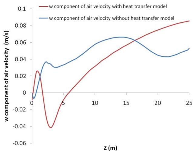
Fig. 15: Comparison of w component of air velocity in z direction at 25m far from source point
