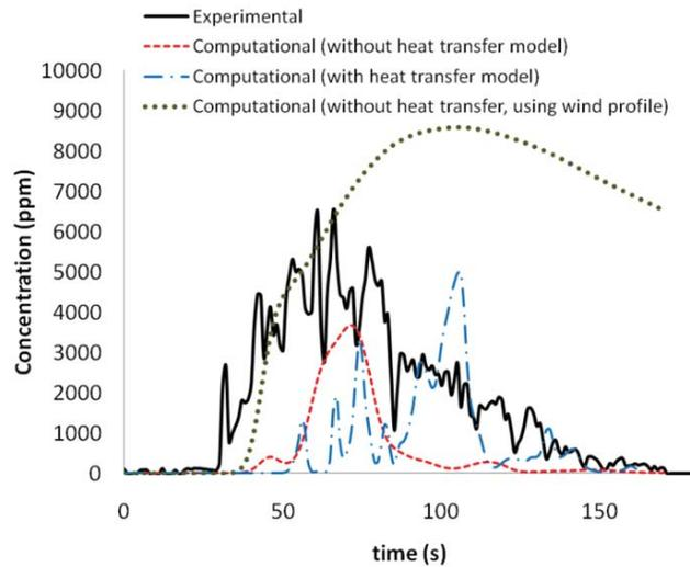
**Fig. 12:** Comparison of experimental and computational results in Kit Fox experiment (trial 3-7) on arc one, at height 1.2m.
