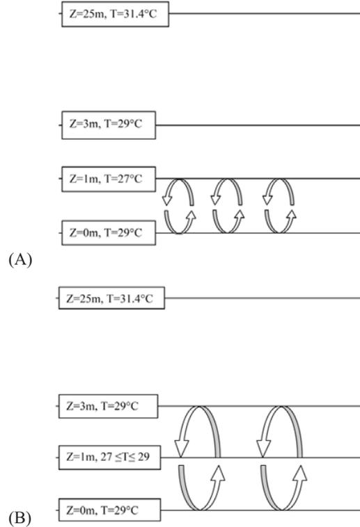
**Fig. 14.a:** Flow recycles in the flat area, b) Flow recycles in the obstacle area
