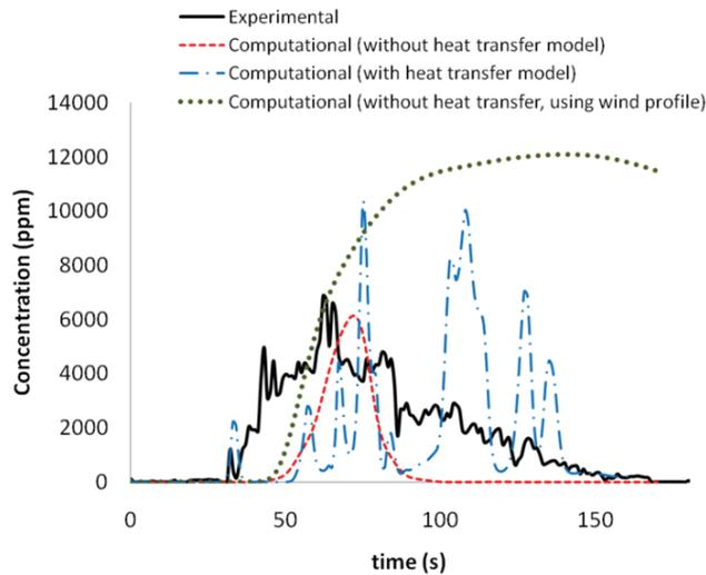
**Fig. 11:** Comparison of experimental and computational results in Kit Fox experiment (trial 3-7) on arc one, at height 0.6m.
