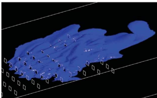
Fig. 16: Gas cloud with 150 ppm isosurface concentration, 100s after gas release. Its volume is equal to 2952.4m<sup>3</sup> and its weight is 72kg.
