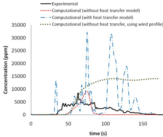
**Fig. 10:** Comparison of experimental and computational results in Kit Fox experiment (trial 3-7) on arc one, at height 0.3m.
