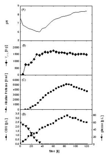
Fig. 6: Cell growth, pH and alkaline protease production during batch cultivation of B. licheniformis in 500 L bioreactor at aeration rate of (1.0 v v<sup>-1</sup> min<sup>-1</sup>).
