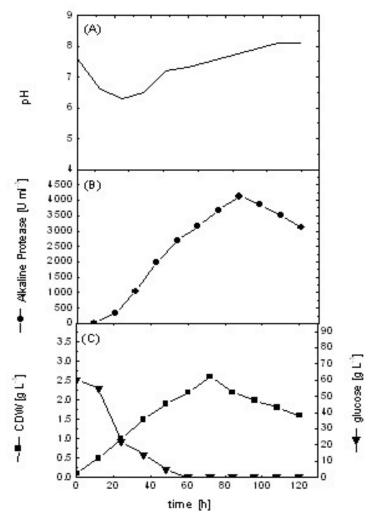
Fig. 4: Cell growth, pH and alkaline protease production during batch cultivation of B. licheniformis in 16 L bioreactor at aeration rate of  $(1.0 \text{ v v}^{-1} \text{ min}^{-1})$ .
