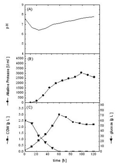
Fig. 3: Cell growth, pH and alkaline protease production during batch cultivation of B. licheniformis in 16 L bioreactor at aeration rate of (0.5 v v<sup>-1</sup> min<sup>-1</sup>.)
