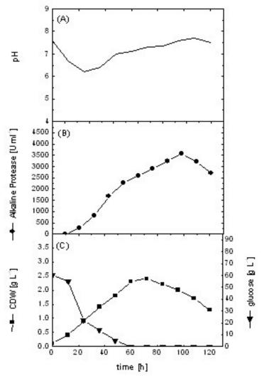
Fig. 5: Cell growth, pH and alkaline protease production during batch cultivation of B. licheniformis in 16 L bioreactor at aeration rate of (2.0 v v<sup>-1</sup> min<sup>-1</sup>).
